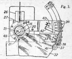
contacts 43 when the waverange is being altered. The device is said to be particularly suitable for mechanical remote control by means of a flexible shaft.
