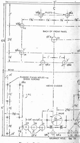
Fig. 4.-Drilling dimensions of the chassis
