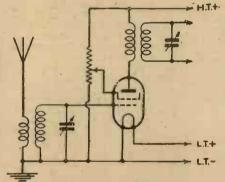
Fig. 3.—Variation of screen voltage for volume control in H.F. stage.
