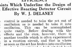
as soon as the set has broken into oscillation as already mentioned a high-pitched howl also sets in, and cannot be stopped until the set has been taken out of oscillation. This, from the fact that you are trying to work on the "threshold of oscillation," and that a howl is set up, gives rise to the term "threshold howl," and also is fairly easily cured.
