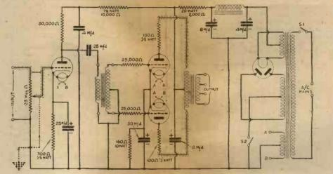
Fig. 3.-Theoretical circuit of the amplifier.
