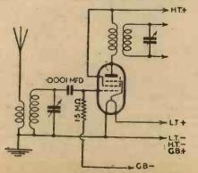
Fig. 5.—Improved circuit for variable-mu control.
