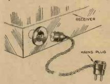
Fig. 3.—" Live" mains connectors should always be insulated. Connectors with open pins or sockets should be "dead" when removed.
