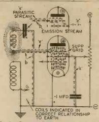
Fig. 2.—Diagram showing the path of electrons in the suppressor-grid system of reaction.
