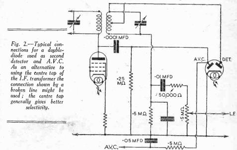
the cathode and H.T.-, were short-circuited, the valve would not be biased. This is because there would be no voltage drop across the resistor. As a result the valve would become excessively hot because of the marked rise in anode current, and would probably be damaged. Additionally, serious distortion would be noticeable.
