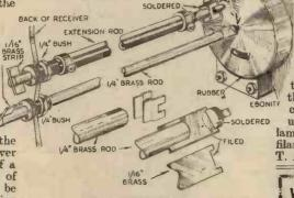
Extension controls for a time-piece fitted to a radio set.
