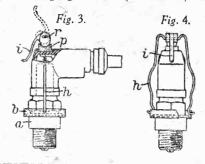
3434.—Standard Telephones & Cables, Ltd., and Earp, C. W.—Mechani-cal modulator for high-frequency waves, particularly for radio beacons utilising two tones. beacons utilising February 23rd.
