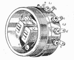
Fig. 2.—How the earpiece was split up and provided with terminals in a further stage of development.
