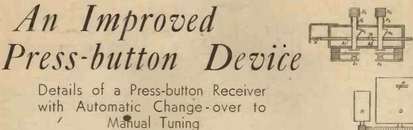
MANY present-day wireless receivers are provided with a control for continuous manual tuning, as well as with push-buttons for selecting one or other of a number of pre-determined stations. In some such cases pressing in a push-button effects the correct setting of the variable condenser by purely mechanical means, while in others the condenser is moved to the required position by means of a motor.
