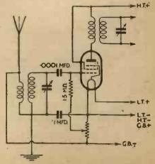
Fig. 6.—A still better form of volume control combined variable-mu and aerial damping.
