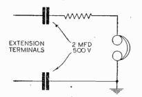
Fig. 1.—One method of phone isolation, with high impedance extension.
