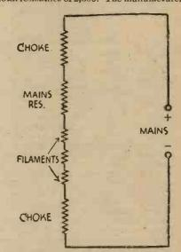
Fig. 4.—The circuit given in Fig. 3 is here shown in simplified form.
