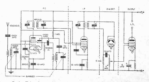
Fig. 1.-Skeleton diagram of a simple S.W. superhet.
