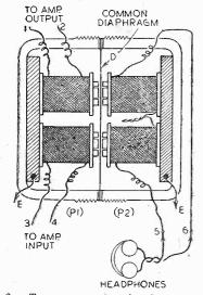
Fig. 3.—Two earpieces combined to pro-ide a similar effect to Fig 1.
