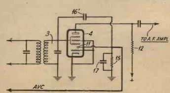
Fig. 3.—In this arrangement the I.F. currents are fed through condenser 16<sup>1</sup>.
