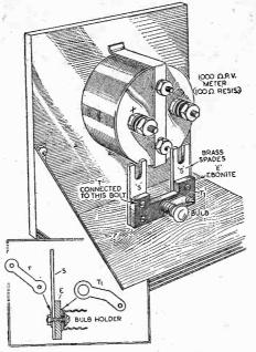
A method of using a torch bulb as a meter shunt.
