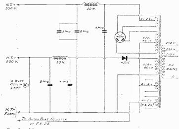
Fig. 3.—Mains section of the receiver, showing the separate H.T. feeds.
