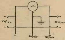
Fig. 1.—Showing the arrangement of the threewire supply system.
