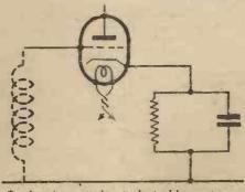
Fig. 6.—Automatic bias is obtained by a resistance and condenser in the cathode lead.
