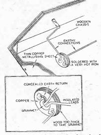
A useful wiring hint for combined wood and metal chassis.
