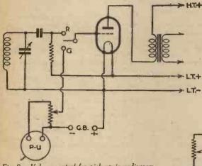
Fig. 8.—Volume control for pick-up in radiogram combination.
