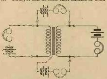
Method of testing a faulty transformer
