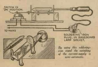
apparatus with which they are to be connected. The resulting arrangement is shown in the accompanying sketches.
