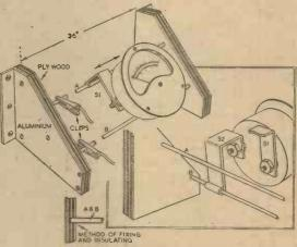
This sliding meter rack facilitates testing work.
