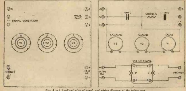
Figs. 4 and 5 .- Front view of panel, and wiring diagram of the bridge unit.
