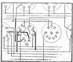
Corrected diagram of part of the value-tester.
