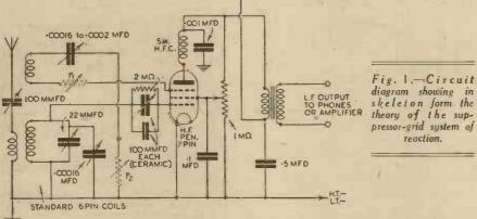
signal injection and reaction, but in recalling these methods to further example the trend in circuit development, the principles adopted with the screen grid should not be confused, theoretically, with the suppressor-grid scheme about to be described, the fundamental difference being evident on considering the action of the screen grid on the characteristics of the valve, particularly in respect of the conversion gain.
