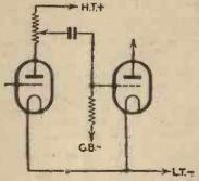
Fig. 9.—L.F. volume control by variable anode resistance.
