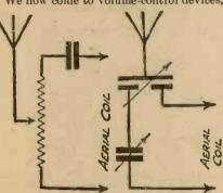
Fig. 1 (Left).—Using a potentiometer form of input control. As an alternative, the arm of the potentiometer may be joined to earth, instead of one end, thus providing a resistance control. Fig. 2 (Right).—A "capacity" potentiometer or differential condenser as input control.
