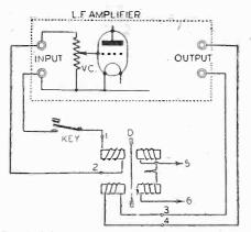
Fig. 4.—Circuit diagram showing the use of the oscillator and keying system.
