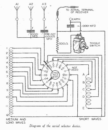
aerial by means of a special filter, which will "lengthen" or "shorten" the aerial as needed. Usually the success of this little device is amazing, and the efficacy of the coil can easily be tested by turning the pointer of the rotary switch to different taps of the coil. There will always be a point where the volume of sound is absolutely sufficient with full rich bass and realistic preservation of the high notes.
