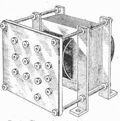
Fig. 1.—Showing how the clamping strips are made and fixed, and a suggestion for a terminal board.
