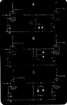
the circuit being arranged that the normal maximum audio voltage across them does not raise the operating point on to the straight portion of the rectifier characteristic curve. Noise peaks cause the rectifiers to work on the straight portion and act as a short-circuit across the output for the duration of the peak.
