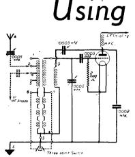
Fig. 1.-For a single tuned circuit receiver, this coil gave very satisfactory selectivity.
