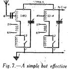
way of obtaining a band-pass circuit using Lissen 5180 and 5314 coils.
