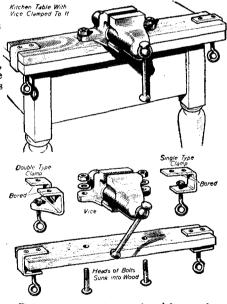
Fitting a vice to a clamping-board for attachment to a kitchen table.
