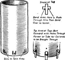
Utilising cardboard cartons for making coil formers.
