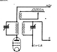
Fig. 4.—A variable-selectivity 1.F. transformer of the type having a tertiary winding.
