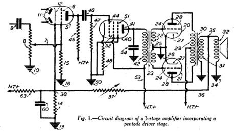
from to be made available for driving the "Class B." stage, and permitting a relatively high gain through the amplifier by reason of the high gain of the pentode stage over the reduction in gain introduced by the high degree of inverse feedback.
