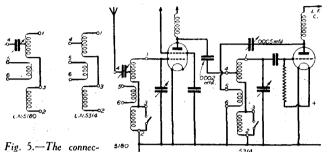
tions for the Lissen coils L.N. 5180 and Fig. 6.—A suitable 3-value circuit for the Lissen L.N. 5314. coils shown on left.
