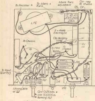
Fig. 3.-Under chassis layout and wiring.
