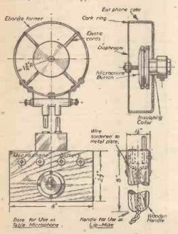
A novel microphone constructed from spare parts.
