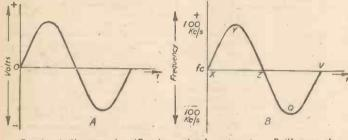
Fig. 1.-A Illustrates the AF voltage plotted against time. B illustrates the conversion of the conver
