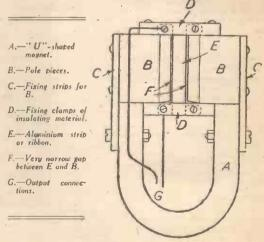
Fig. 2 .- Details of a ribbon microphone.
