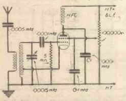
Fig. 1.—Outline circuit of a cathode-coupled regenerative detector. It should be compared with the circuit shown in Fig. 2. Values shown are applicable to a short-wave receiver. Valoes
