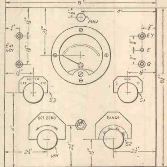
Fig. 4 .- Panel layout and drilling measurements.
