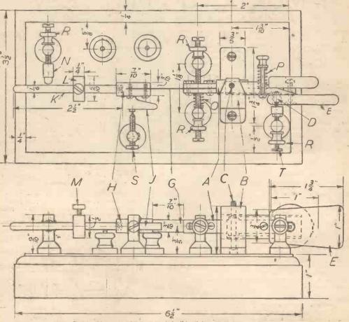
Fig. 3 .- Plan and side elevation of the "bag" key described in the text.
