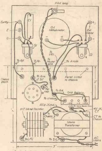
Fig. 2 .- Panel and top of chassis layout and wiring diagram.
