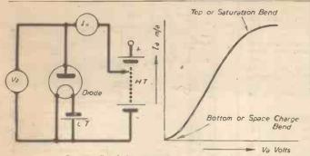
Fig. 13.—The la/Va characteristic curve of a diode.
