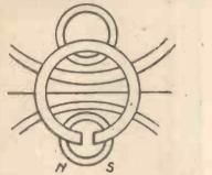
Fig. 5 .- Diagram indicating leakage by atmospheric paths.
