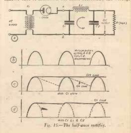
direct current, thus the fluctuations produce an alternating voltage across  $L_1$  which forces alternating current around the circuit  $L_1$   $C_1$  .  $C_2$ , thus wasting the energy of these fluctuations.
