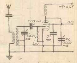
Fig. 2 .- A tetrode value used in a conventional Reinartz reaction circuit.
