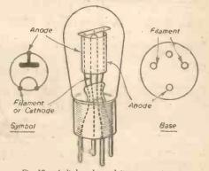
Fig. 12 .- A diode value and its component parts.
