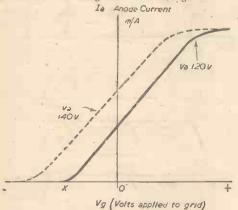
Fig. 18 .- A typical la/Vg characteristic curve of a triode.
