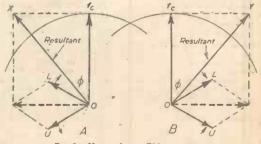
Fig. 5.-Vectors for an FM transmission.
