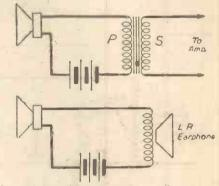
Fig. 4.-Connections for carbon microphones.
