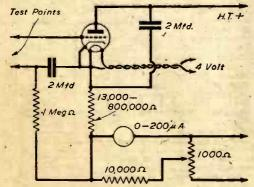
Fig. 4.—Circuit of an H.F. valve voltmeter using an Osram type A.577 valve.
