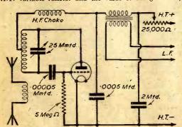
Fig. 1.—A self-quenching super-regenerative detector, suitable for U.S.W. reception.
