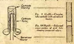
it is frequently plated with rhodium—a rare metal of the platinum group—and it is generally necessary to polish the grid hole as shown in Fig. 10. This is principally to ensure that no fine airborne fluff will adhere to the edges and obstruct the beam.
