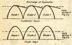
Fig. 3.—Output voltage wayeforms of a full-wave rectifier with a condenser and choke output.
