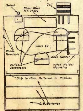
Fig. 3.—Rear view of the interior of the receiver, showing how the valve is mounted.
