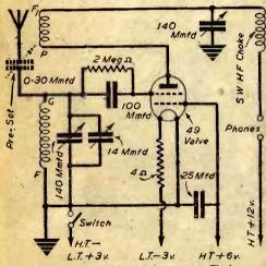
Fig. 1.—The theoretical layout of the receiver. The letters on the coils refer to pin connections on holder. See Fig. 4.
