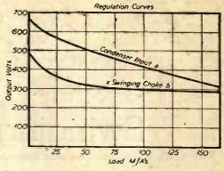
Fig. 4.—Regulation curves of two types of power pack.
