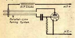
Fig. 3.—Resonant—or parallel—line tuning, which is most satisfactory for use with ultra-short and micro-waves.
