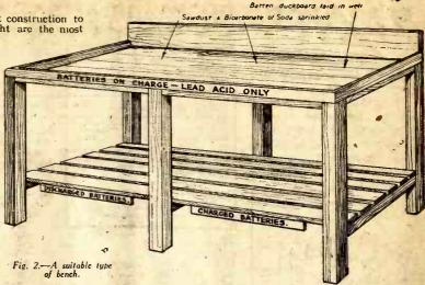
charging room for dealing with lead batteries only, but with provisions made for extending to alkaline. The rectifier and A.C. switchgear is installed in a separate compartment, which is also utilised as an office and store. One pair of cables feeds two charging panels, each of which has four sub-circuits, e.g., sets of terminals, each set controlled by a separate variable resistance. Fig. 3 illustrates this name! illustrates this panel.
