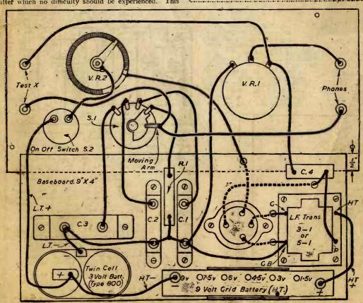
Fig. 6.-Layout and wiring of the component parts.
