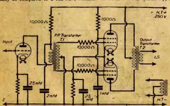
Fig. 1.—A tetrode push-pull stage following a triode amplifier. The latter may be the triode portion of a double-diode triode.
