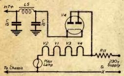
Fig. 9.—(Above) Modifications for low anode voltage valves.
