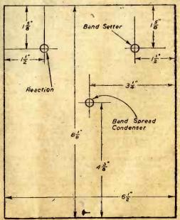
Fig. 2.—At the top is shown the dimensions for the horizontal panel. The lower diagram is that for the main or vertical panel.
