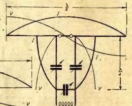
maximum results with the wavelength concerned. Loading coils, however, are not to be desired, because of the reduction of the aerial's overall efficiency.
