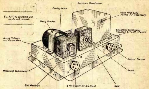
of a can made from a piece of old tinplate and bolted securely to the base. For the battery and output connections, two old valveholders were used, and the connections were through four-pin adapter-plugs.
