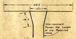
Fig. 77.—The use of a non-resonant feeder with a \(\lambda/2\) (approx.)
