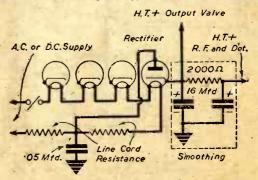
Fig. 2.—A typical H.T. smoothing circuit as used in midget A.C.iD.C. receivers.
