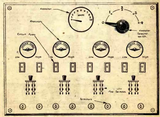
Fig. 3.—A four-circuit charging panel.
