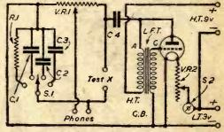
Fig. 4.—The circuit of the resistance and capacity bridge described by the writer.
