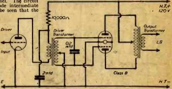
Fig. 2.—Driver and Class B stages of a battery amplifier suitable for an output in excess of one watt.
