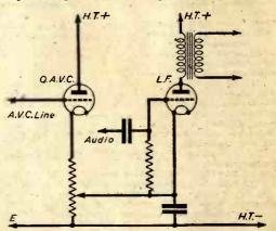
Fig. 5.—This diagram illustrates the principle of quiescent automatic volume -control.
