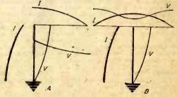
Fig. 72.-A, "Inverted L" aerial. B, "T" type aerial. Fig. 70.—(Left) A, Travelling waves; B, Standing waves: C, Current and voltage distribution.
