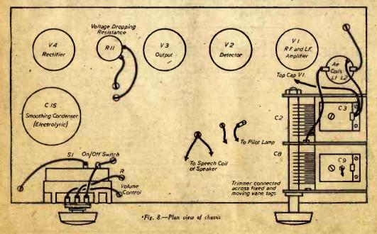
component position for both underside and top of the chassis, the tubular condensers and resistances have been decreased in size to give greater clarity. All resistance except R<sub>11</sub> may be \( \frac{1}{2} \) w.
