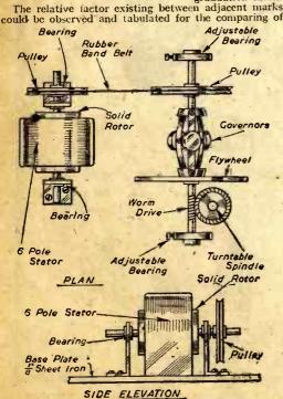
A converted cycle dynamo used as a gramo-motor.
