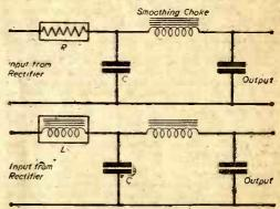
Fig. 2.—(a) (upper) Zero inductance is represented by R—the D.C. resistance of the winding. (b) (lower) The same choke shown as an inductance, L.
