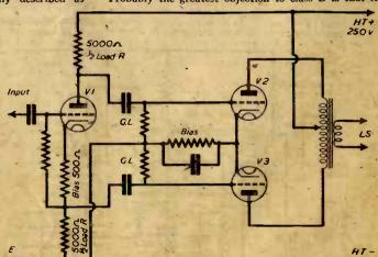
Fig. 4.— Outline circuit of a paraphase amplifier where value VI takes the place of a push-pull transformer, and acts as a phase-splitter, while V2 and V3 behave as normal push-pull values. The values shown are purely nominal, and are intended primarily to show that resistors of equal value are used in anode and cathode circuits.
