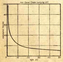
Fig. 1.—Curve showing the relationship between the D.C. component and inductance of an iron cored choke.
