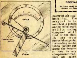
A simple Magnetometer.
