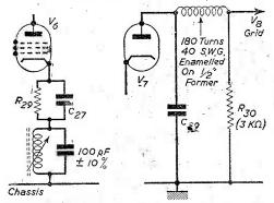
Fig. 1.— The sound trap is included in the cathode lead of the last I.F. valve.
