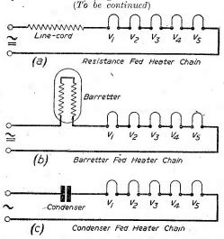
Fig. 1.—The basic feed methods for a series heater chain.
