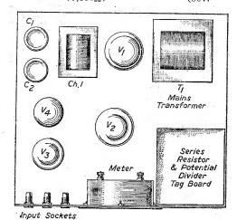
Fig. 3.—Chassis layout.
