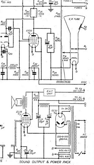
are successively decoupled so that a gradually increasing H.T. is applied from stage to stage up to the output.
