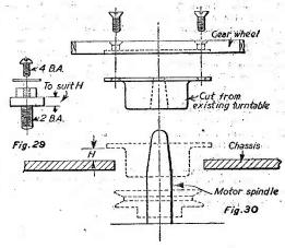
Figs. 29 and 30.—The idler pin, and details of the positioning of the gear wheel and driving pulley.
