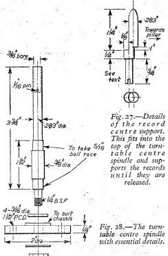
do not slide as easily with the weight of the upper records on them. The cranked spindle can be mounted two ways. The correct way is with the cranked portion towards the table. To get the pin in the centre spindle in line so that the slot in the bottom of the cranked spindle locates the crank in the correct position it will be necessary to rotate the centre spindle.
