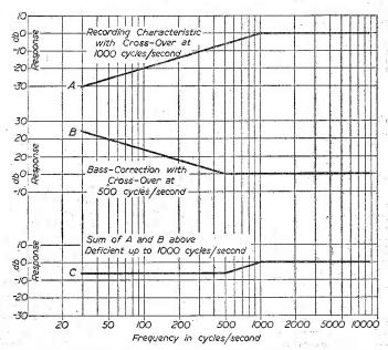
Fig. 3.—Showing the effect of play-back with the wrong bass-correction characteristic.
