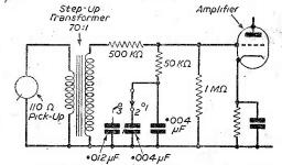
Fig. 5.—The circuit of Fig. 4 modified to give any of three characteristics. Boost is available for cross-over frequencies of 250, 500 or 1,000 cycles/second.
