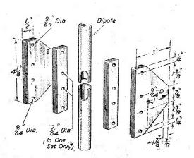
Fig. 4.—Essential details of the clamp. Two sets of these are required.
