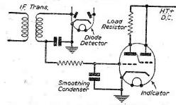
Fig. 5.—In this circuit delayed A.V.C. is utilised.
