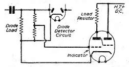
Fig. 4.—Another circuit with diode control.
