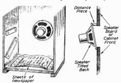
Figs. 1 and 2.—Cabinet resonance may be modified or reduced, as shown here.
