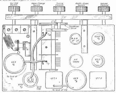
Fig. 4.—Top of chassis view of the tuner.
