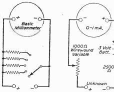
Fig. 7.—How shunts may be switched for multi-range milliammeters.
