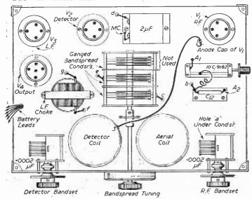
Fig. 3.—Above chassis layout and wiring details.
