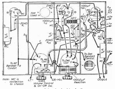
Fig. 4.—Below chassis wiring details.
