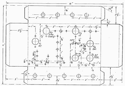
Fig. 2.—Drilling and cutting details of the chassis.
