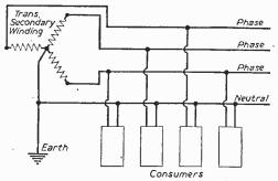
Fig. 1.—Three-phase, four-wire system for A.C.
