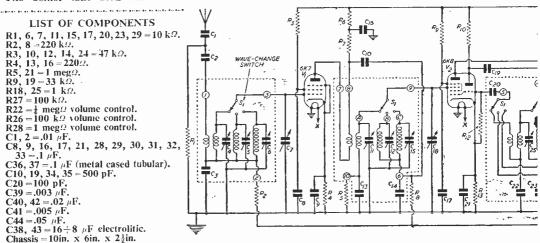
Fig. 1.—Theoretical circuit of the tuner unit. The components within
