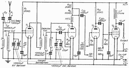
Fig. 1.—Theoretical circuit of the receiver with components numbered as in the T/R9.
