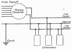
Fig. 2.—Three-wire D.C. supply.
