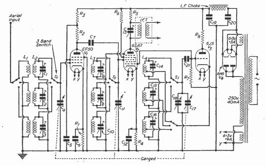
Fig. 1.—Theoretical circuit of the converter.
