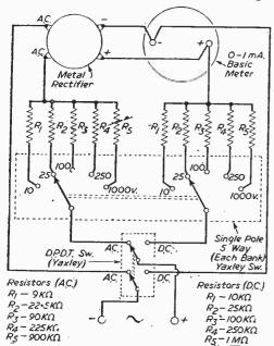
Fig. 6.—Comprehensive circuit, with switching, of A.C./D.C. multi-range voltmeter. Note: D.C. resistor values are actual, A.C. values approximate (before calibration).
