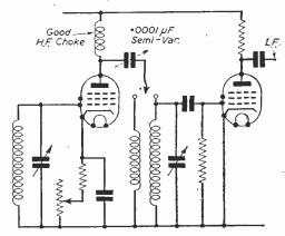
Fig. 5.—Choke-coupled H.F. stage showing how variable selectivity may be added.
