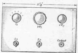
Fig. 3.-Layout of panel.
