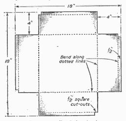
Fig. 2.—Details of the chassis.
