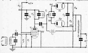
Fig. 17.—A frequency demodulator consisting of an amplitude limiter and a phase discriminator,
