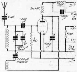
Fig. 2.—Simple one-valve converter.
