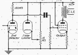
Fig. 2.—Simple clipper circuit.
