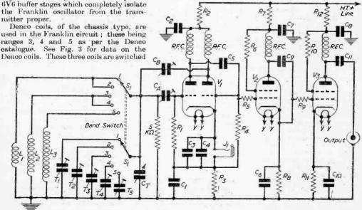
Fig. 1.—Circuit of the 5-band V.F.O. unit.
