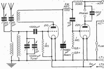
Fig. 1.—Theoretical circuit of a simple two-valver-
