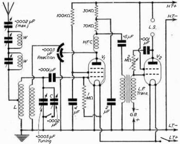
as the near and powerful Fig. 1.—Theoretical Circuit. Note the wavetraps W, the coil L, and the cones.
