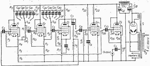
Fig. 1.—Theoretical circuit of the oscillator.
