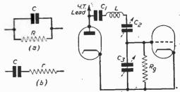
Fig. 13 (a) and (b). $\rightarrow$ These two circuits are actually identical.
