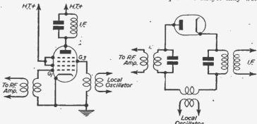
at fringe areas before the signal Fig. 13.—Two types of mixer circuits for obtaining the heterodyne beat is fed to the demodulator.
