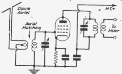
Fig. 12.—The functional circuit of a V.H.F. amplifier stage.
