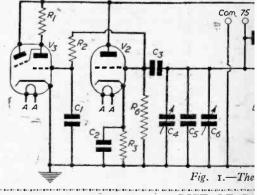
LIST OF CO R4-30KΩ. -1.5 KΩ 5W. C1, C2, C3 and C7 -5 pF variable. -520 pF (see te R1, R2 and R6-1M2 -55 turns of wire wound in a single L2-60 turns of wire wound at other
