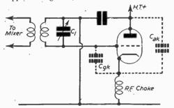
Fig. 14.—The modified Colpitts oscillator circuit—suitable for use as the local oscillator of a V.H.F. receiver. The anode is effectively earthing at R.F. so that CI may form part of a two- or three-gang variable capacitor.
