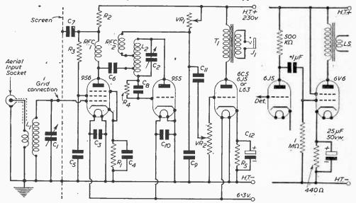
Fig. 1.—Theoretical circuit and alternation L.S. output,
