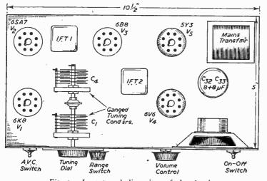
Fig. 2.—Layout and dimensions of the chassis.
