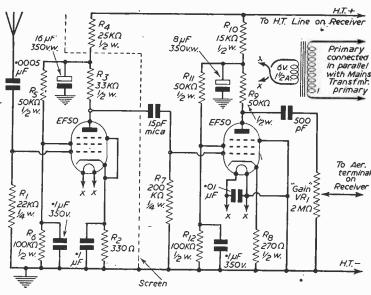
The circuit of the pre-amplifier. No separate list of parts is given as all details are marked on the circuit.
