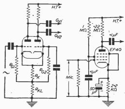
Fig. 6.—The phase inverter stage.
