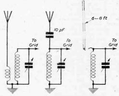
Fig. 1—An un- Fig. 2—Another Fig. 3—A tuned tuned aerial, form of untuned aerial.
