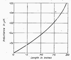
Fig. 16.—The inductance of a straight 20 s.w.g. copper wire.
