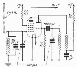
Fig. 4—Tuned aerial circuit in a frequency changer stage of a superhet or S.W. converter.
