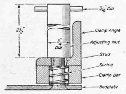
Fig. 2.—The spring-loaded clamp.
