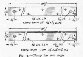
between clamp bar and bed for different thicknesses of materials.
