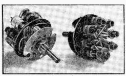
The midget coil turrets as supplied by Stern Radio Ltd.
