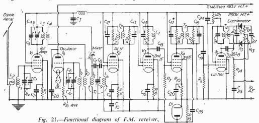
the adjustment of L5 and L6, then the second peak at 4.6 Mc/s should be tuned by means of capacitor C9. These adjustments are somewhat interdependent and, if a large movement is necessary, should be repeated until the correct bandwidth is obtained.
