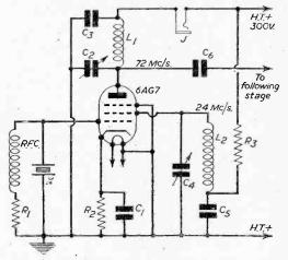
Fig. 1,—Oscillator circuit for harmonic crystals.
