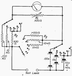
Fig. 4.—Circuit of the complete ohmmeter.
