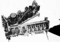
A 15 valve (6V6, VU39A, 4/SP61, 4/EA50, 2/EF54, EF50, EC52, VU111) dual chassis radar receiver for 223 Mc/s with 13 Mc/s IF, strip R.F. section, high cycle power section antenna switch, relay, etc., etc.,
