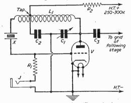
Fig. 2.—Squier crystal oscillator circuit.
