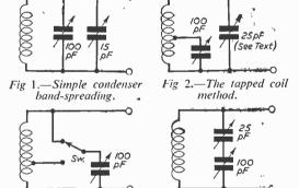
Fig 3.—Tapped or full coil. Fig. 4.—The series method.
