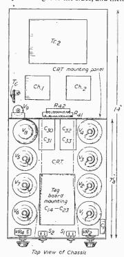
Fig. 5.—Views of the chassis showing layout of essential parts.
