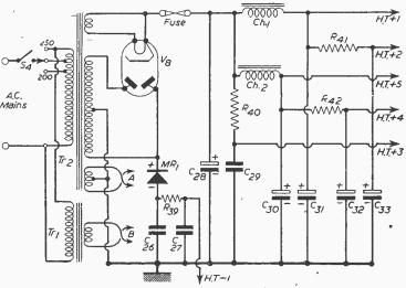
Fig. 2.—Theoretical circuit of the power supply section.
