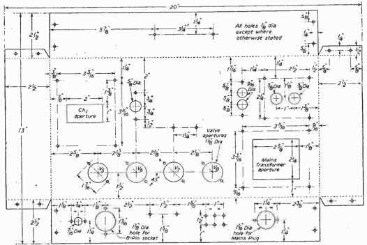
Drilling details for the amplifier and power pack chassis.
