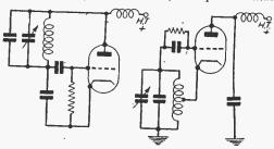
Fig 3. — The Colpitts oscillator.
