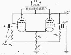
Fig. 1.—Basic circuit of the Schultz phase-splitter.
