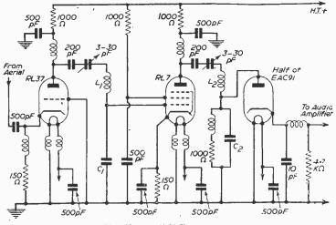
Fig. 49 — A V.H.F. converter.
