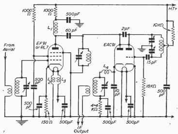
Fig. 54.—Another self-quenched super-regenerative arrangement.
