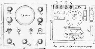
Fig. 3.—Panel and C.R.T. mounting details.
