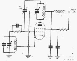
Fig 6.—Neutralised anode circuit form of "electroncoupled" oscillator.
