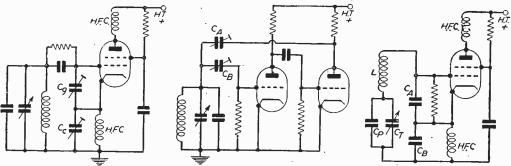
Fig 7.—Condenser tap version of the "electron-coupled" oscillator. This is not to be confused with the similar Clapp circuit. C<sub>2</sub> and C<sub>6</sub> are cathode tapping condensers of, say, 100 pF, and 500 pF, respectively.
