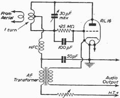
100 $\Omega$ . Full-scale deflection Fig. 53.—One form of super-regenerative circuit. be detected.
