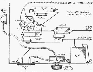
Fig. 2.—Wiring diagram of the 6J7 stage.
