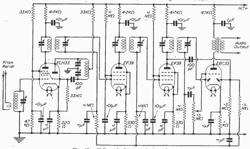
Fig. 48.—H.F. end of a complete receiver.
