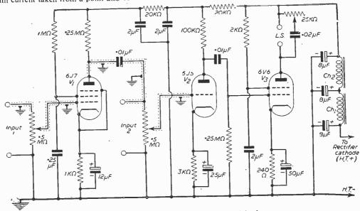
Fig. 1.—Amplifier circuit showing screened leads, etc.
