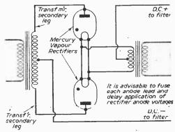
Fig. 1.—Basic circuit of a rectifier unit.
