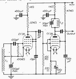
Fig. 47.— $L_1$  consists of  $6\frac{1}{2}$  turns 18 s.w.g. on a  $\frac{1}{2}$ in. former, tapped 2 turns from the "hot" end.  $L_2$  consists of 2 turns 18 s.w.g. on a  $\frac{1}{2}$ in. former (this coil can be self-supporting).
