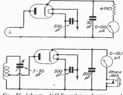
Fig. 56 (above).—V.H.F. valve voltmeter, and Fig. 57 (below).—A wavemeter for V.H.F. work.
