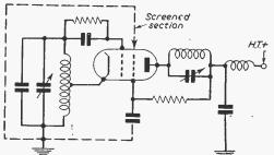
must be replaced by a Fig. 5.—"Electron-coupled" form of the grounded suitable negative coefficient anode Hartley. The oscillator output is coupled from ceramic condenser. Without the screen-enclosed oscillator section via the electron going into details, the stream, if a fully screened valve is used.
