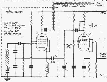
Fig. 1.—Basic N.B.F.M. V.F.O.-reactance modulator circuit.
