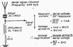
Fig. 6.—The acceptor circuit.
