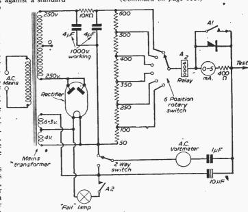
Circuit of the condenser test set.
