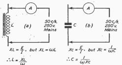
Fig. 1 (a) and (b).—Method of measuring the value of L or C,
