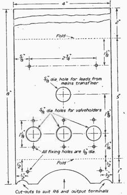
Fig. 3.—Drilling diagram for chassis.
