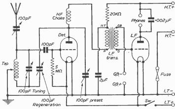
Fig. 1.—Theoretical diagram of a 2-valve Hartley Circuit.
