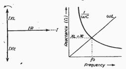
Fig. 4. (Left)—R, XL and Xc in series. Fig. 5. (Right)—At one point foXL = Xc.
