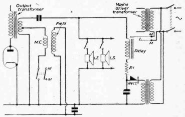
Circuit diagram of the remote control system.
