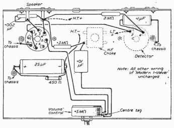
Components and wiring for the L.F. stage.
