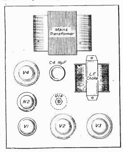
Fig. 5.—Chassis layout.
