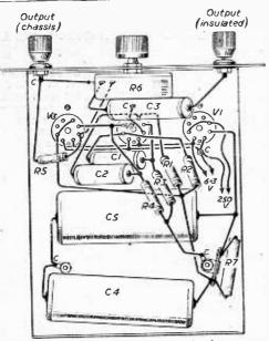
Note: Mains transformer is on top of chassis Points marked C are connections to chassis Fig. 2.—Wiring diagram of the High Speed Fault
