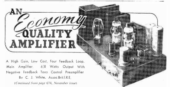
HILST being pleased with this result it was at once apparent that still more improvement could be made. The gain of VI was increased to 520 times: the feedback in the main loop increased to 23db and the input requirement brought down to 0.4 volts R.M.S. for 6 watts output, and it is with these constants that the amplifier is now put forward. The reduction of the input requirement is particularly useful in that whilst maintaining the very high quality it enables the require-
