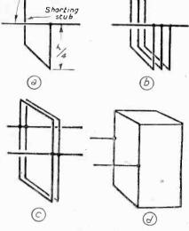
Fig. 3(a).—This stub has no effect on the line since the open end is of high impedance. (b) More stubs added to line. (c) More added edge to edge. (d) If the number of stubs is increased indefinitely and placed into contact, a metal tube, ½2 high results.
