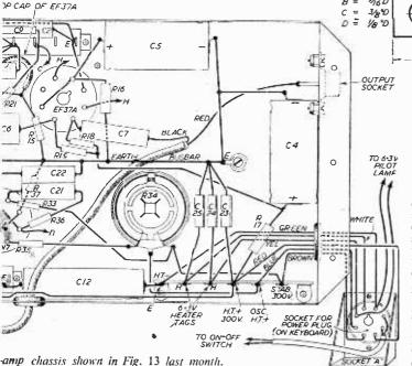
pected that a single mains transformer could be used for this as well as the remaining H.T. and L.T. supplies. Accordingly, a separate heater supply is provided and in the original a shelf was placed towards the top of the main organ body,
