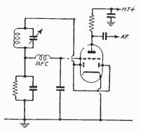
Fig. 1.—Typical half-wave detector—Diode anodes strapped together.
