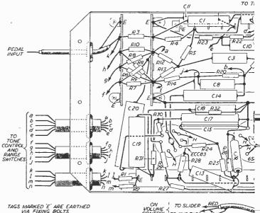
VALVE HEATER LEADS MARKED H' ARE TWISTED AND TAKEN TO 6.3V TAGS
