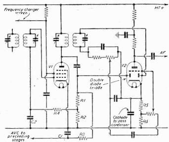
Fig. 3.—Typical circuit using a D.D.T. valve.
