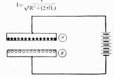
Fig. 39.—Dielectric strain in charged condenser.
