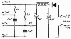
Fig. 2. - Intermediate voltages and direct operation.
