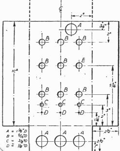
Fig. 17.—Chassis cutting and drilling data for the units shown on page 31.
