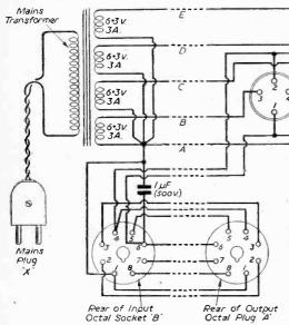
Fig. 18.—Theoretical circuit of the sub-power unit.
