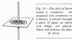
Fig. 35.—The field of force round a conductor. An insulated wire connected to a battery is passed through a piece of paper on which iron filings are placed. These will indicate the lines of force.
