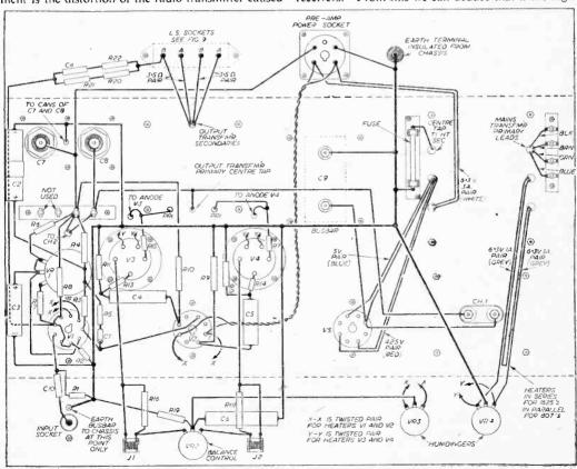
Fig. 12.-Wiring details for the amplifier.
