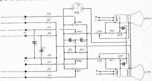
Fig. 3.—The cathode-ray tube unit.
