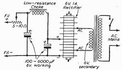
Fig. 3. -L.T. circuit for 1.4-2.0 volts.
