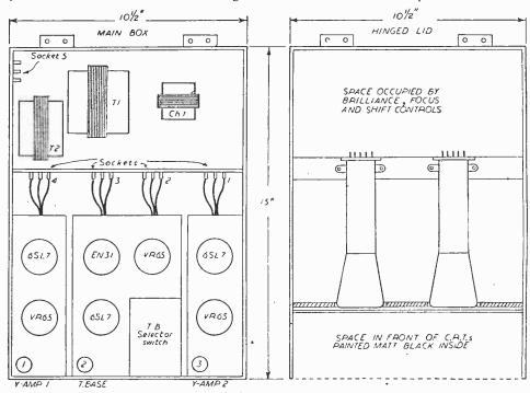
Fig. 1.—General layout of main components.
