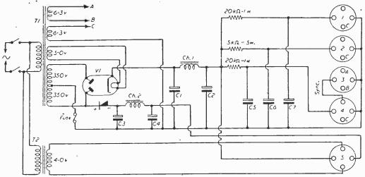
Fig. 2.—The power pack—C1 to C7 inclusive are 8nF 450 r.w. electrolytics.
