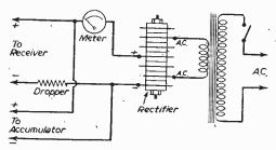
Fig. 6.—Trickle charger with dropper for 1.4v.
