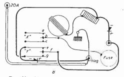
Fig. 13b.-New wiring denoted by heavy lines.
