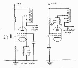
Fig. 1 (left).—The tapped primary winding of a mains transformer enables some degree of load matching to be effected.
