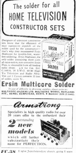
FC.38 8 valve Superheterodyne chassis, giving 8 watts push-pull output with negative feedback and separate BASS and TREBLE ht controls, WAVE RANGE : 16-50 metres, 190-550 metres and 1,000-2,000 metres. PRICE : £23 13s. including tax.
