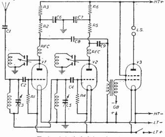
Fig. 1.-A simple dual-channel receiver.
