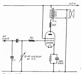
Fig. 2.—H.F. stoppers are shown here at R1 and R2.
