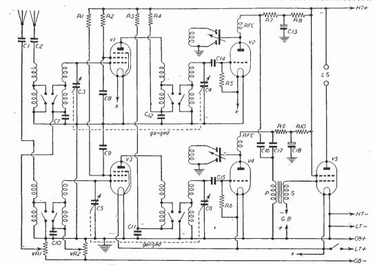
Fig. 3.—Another type of dual-channel receiver.
