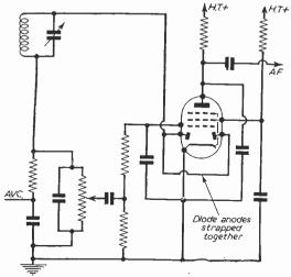
Fig. 2.-Basic circuit showing half-wave detection, A.V.C. and fixed bias amplifier.
