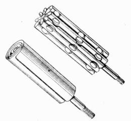
Fig. 50.—Two typical anode designs used in electrolytics.
