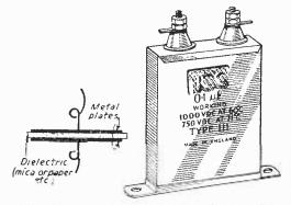
Fig. 45.—Principle of a fixed condenser and a typical "paper" type fixed condenser.
