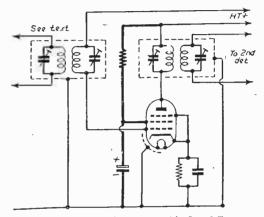
Fig. 4.—Decoupling the screen-grid of an I.F. stage.
