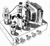
LOOPS with 15 db in the main loop from output transformer to voltage amplifier. Frequency response +3 db. 50-20.000 c.p.s. HUM and DISTORTION LESS THAN 0.5
