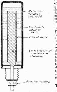
Fig. 49.—Details of construction of a typical "wet" electrolytic condenser.
