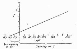
Fig. 2.—A graph of various readings at different frequencies on a "Q" meter in checking the selfcapacity of a coil.
