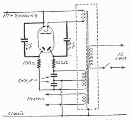
Fig. 1.- The heavy lines show the modifications to be made to avoid modulation hum.
