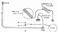
Fig. 13a.—The part of the wiring to be altered.
