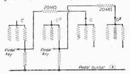
Fig. 25.—Details of circuit for obtaining the pedal notes.
