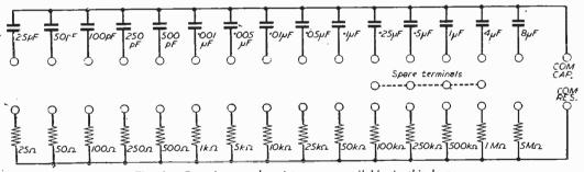
Fig. 6.-Capacitors and resistors are available in this box.
