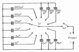
Fig. 2.—A switched version of a capacitor selector.
