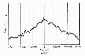
Fig. 2.—Typical recording of the transit of a radiostar, indicating "scintillation."
