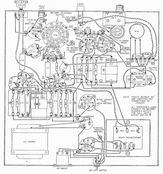
Fig. 5.—Wiring diagram of the amplifier. Note that R24 should be  $220\Omega$  and not 220K as shown in the list of parts.
