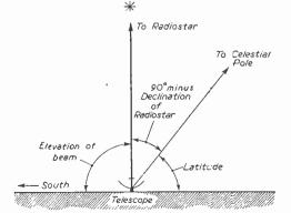
Fig. 1.—Setting up a radio-telescope : The declination of the area of the sky investigated depends on the elevation of the beam and on the latitude of the place of observation.
