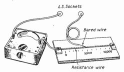
Fig. 91.—A simple output measuring device. The resistance may be made up by using bare resistance wire wound over a thin former.
