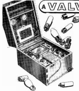
THE tester has been designed for simple operation, providing a very useful portable instrument. For simplicity A.C. volts are used for the main supplies, and on all tests the meter indicates the average of the current pulses resulting from the self-rectification of the valve under test.
