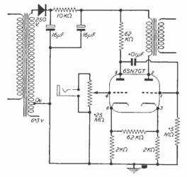
Fig. 1.—Basic theoretical circuit.
