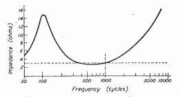
Fig. 33.—Impedance curve of a typical moving-coil speaker, nominally 3 ohms.
