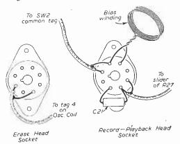
Fig. 2.—Details of the head connecting leads shown below.
