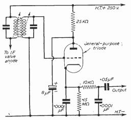
Fig. 6.—The well-known infinite impedance detector.
