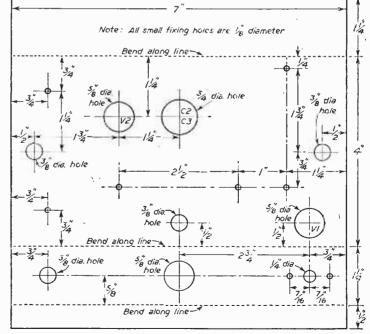
Fig. 37.—Chassis drilling diagram for A.C. amplifier (Fig. 36). Note that the  $\frac{3}{4}$  holes are for growthmets.
