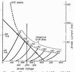
*Fig.* 34.—*Characteristic of* 6*A*Q5; 19*A*Q5; 6*BW*6.
