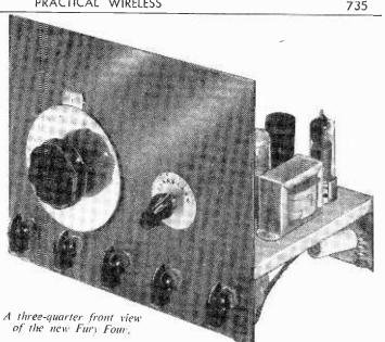
products by Denco, and they are easily fixed by means of their one-hole fixing nuts, and have an iron-core for matching. They are tuned by a 310 pF condenser instead of the usual 500 pF, and this improves performance on the short waves. It will be seen in the circuit diagram that a three-way switch is used for each coil (these being in the form of a six-position, three-way Bulgin component), and instead of using a
