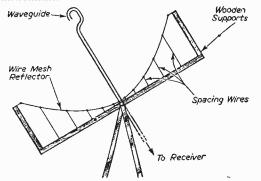
Fig. 3.—Cross-section through a parabolic reflector with waveguide for the reception of radiations in the microwave region.
