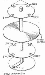
Fig. 6.—How the switch assembly is made up.
