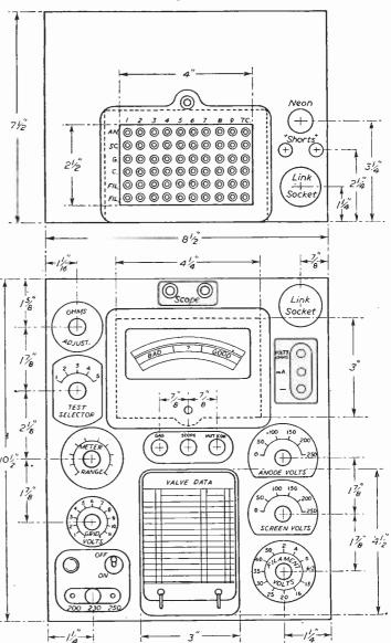
Fig. 4.—Details of the panel layout. See the illustration on page 714.
