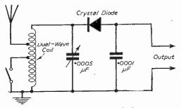
Fig. 1.-A simple crystal diode tuner.
