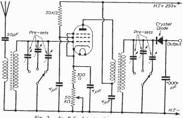
Fig. 3 .- An R.F. detector Pre-set tuner.
