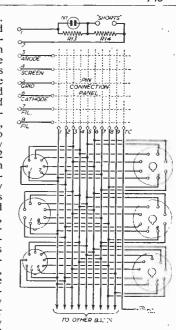
Fig. 2.—Wiring to the valveholders,
