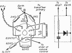
Fig. 2.—Wiring layout and suitable probe unit.
