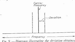
Fig. 9. — Diagram illustrating the deviation obtained in F.M.
