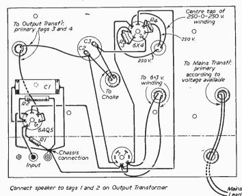
Fig. 38.—Wiring diagram for the Fig. 36 circuit.
