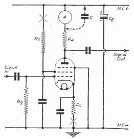
Fig. 9.—Always make current tests at a low signal potential point in the circuit.
