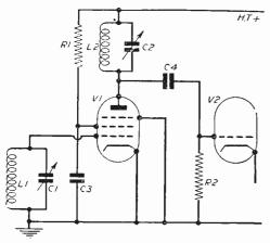
Fig. 48.—Basic R.F. amplifying circuit.
