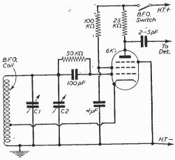
Fig. 1.—A typical B.F.O. stage.
