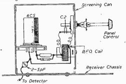
Fig. 6.—A typical B.F.O. stage layout.
