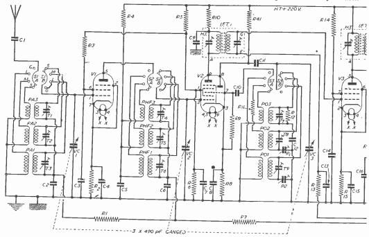
Fig. 1.—Main circuit diagram—excluding the power pack which will be given next month. A full list of con-
