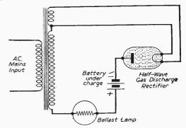
Fig. 2.—This shows a half-wave circuit.
