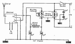
Details of a converter power supply.
