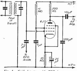
Fig. 4.—Grid detector with BFO input.
