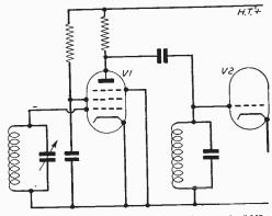
Fig. 50.—Tune.l circuit transferred to grid of V2.
