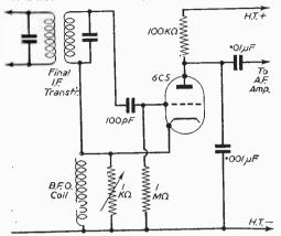
Fig. 5.—A cathode-coupled det./B.F.O. stage.
