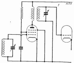
Fig. 51.—Basic transformer—coupled circuit.
