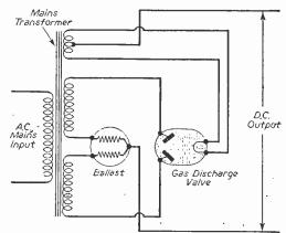
Fig. 1.—The full-wave circuit with centre-tapped filament,
