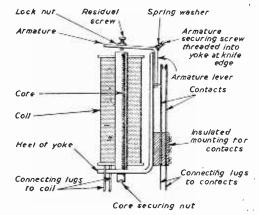
Fig. 1.—Cross-section of a typical relay. The coil lugs pass through holes in the heel of the yoke. An extension on the moving contact nearest the voke bears against an insulated inset on the armature lever.
