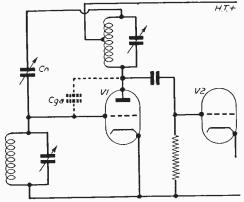
Fig. 49.—Method of neutralising grid anode capacitance.
