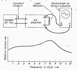
Fig. 49.—A method of checking the frequency response of an A.F. amplifier.
