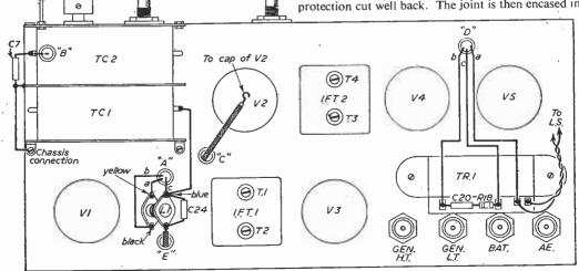
Fig. 5.-Top chassis view of the receiver.
