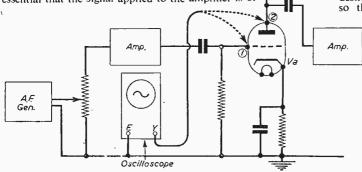
Fig. 48.—Showing a method of checking stage gain.
