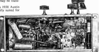
An underside view of the receiver showing the wiring.
