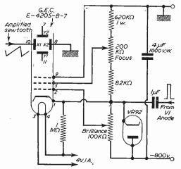
Fig. 7(a).—Power supply for 2½in. tube, showing flyback suppression.
