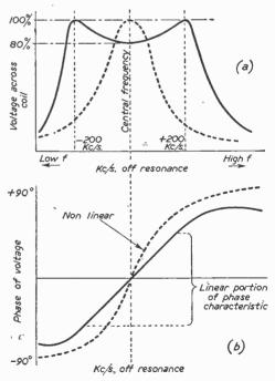
Fig. 2.-I.F. response curve required (a) and resulting phase characteristic (b).
