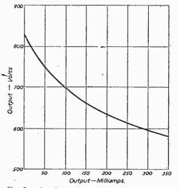
Fig. 5. — Regulation curve of a 600-volt condenser input circuit power pack.
