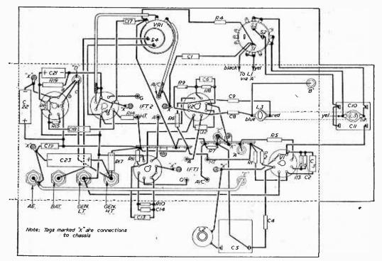
Fig. 4.-Wiring diagram of the receiver section,
