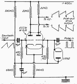
Fig 7(b). — Push-pull deflection with flyback suppression.
