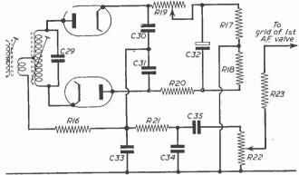
Fig. 4.—Circuit of the F.M. detector stage.
