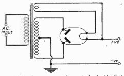
Fig. 2.—In low-power packs a single double-diode rectifier is commonly used.
