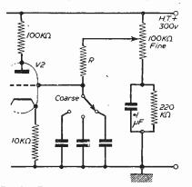
Fig. 6.—Fine and coarse scan-time controls.
