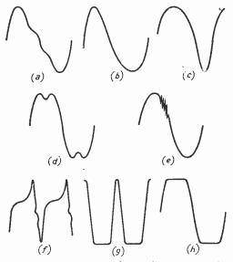
Fig. 47.—Distortion waveforms often encountered in A.F. amplifiers.
