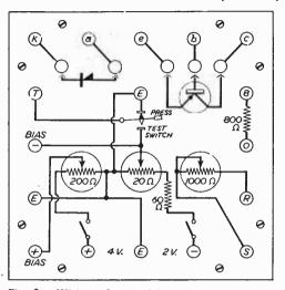
Fig. 2.—Wiring of a diode/transistor test panel.
