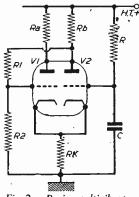
Fig. 2.—Basic multivibrator circuit.
