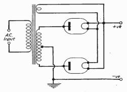
Fig 1. --- The full-wave rectifying circuit.
