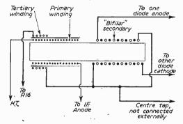
Fig. 5.—Details of the discriminator transformer. Wiring details are on page 756.
