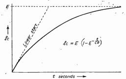
Fig. 1.—Build-up of voltage across a condenser.
