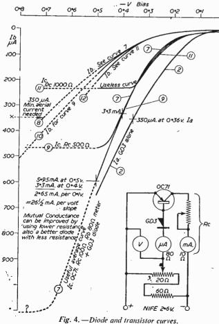
(4) Ib input curve. At -0.3 volts it shows that the transistor requires 225  $\mu$ A for an output of 9.45 mA and curve two shows that the diode passes 250  $\mu$ A, enough by a small margin.
