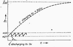
Fig. 5.—Scan and flyback as part of charge and discharge characteristic.
