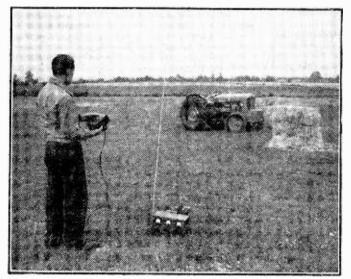
A radio-controlled tractor at work.
