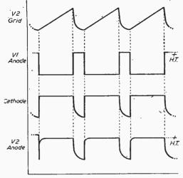
Fig. 3.-Multivibrator waveforms (not to scale).
