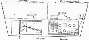
Fig. 7.-Plan and sile view (above) of the method of housing the receiver.
