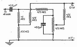
Fig. 4.—A continuously variable bass boost circuit.
