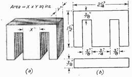
Fig. 6.—Core area and suitable laminations.
