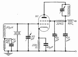
Fig. 5.—A more elaborate circuit for "rubberising" a crystal.
