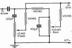
Fig. 5.—Separate controls for treble and bass.
