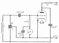
Fig. 75—A grid-dip oscillator using a Colpitts oscillator.
