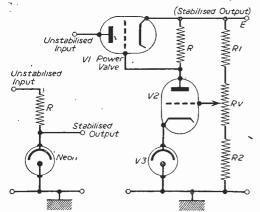
Fig. 1.—Neon stabiliser. Fig. 2.—Simplified series regulator.
