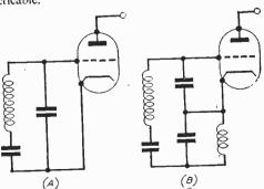
as it decreases the effective airgap includes the effect of the Fig. 2.—The similarity of the equivalent crystal capacity across the crystal. A holder plate capacity and circuit (a) to the Clapp-Harries oscillator circuit
