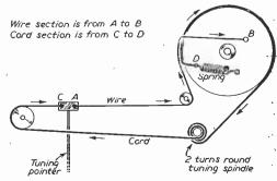
Fig. 4.—Details of the Cord Drive for the Tuning.
