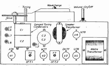
Figs. 2 and 3.—Above and below chassis layout with main components identified.
