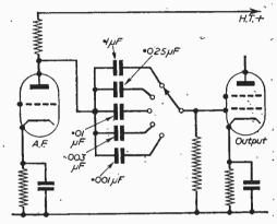
Fig. 2.—Bass cut by coupling capacity selections,
