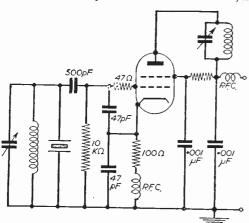
Fig. 6.—A cathode tap variation upon the basic circuit of Fig. 5.
