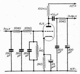
Fig. 7.—Steep cutting H.F. filter.
