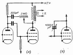
Fig. 6.—Using negative feedback to reduce top.
