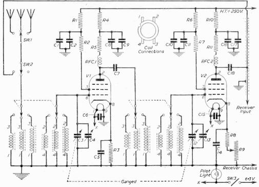
Fig. 1.—Theoretical circuit of the pre-selector.
