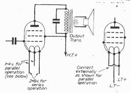
Fig. 5.—Basic circuit for output, using 2.8 volt filament valves.
