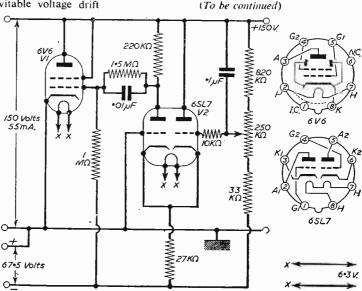
Fig. 5.—The circuit of a practical stabiliser.
