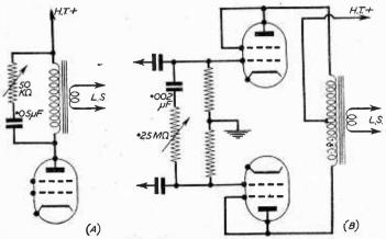
Fig. 1.—Two simple top-cut controls.
