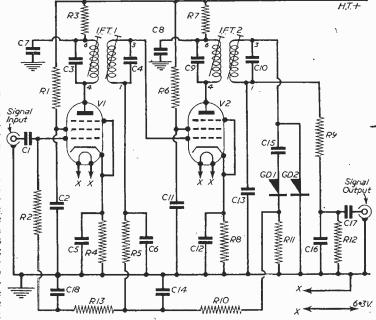
Fig. 14.—1.F. circuit diagram.
