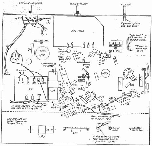
Fig. 4.—Wiring details and main component layout.
