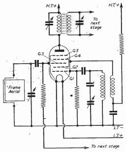
Fig. 1.—Basic circuit of frequency changer for battery miniature valves.
