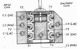
Fig. 5.-Details of the coils and trimmers.
