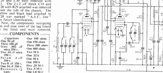
50 pF and 100 pF capacitors, and the 0.1 M $\Omega$  and 0.5 M\O resistors were soldered to this six-way tag strip. The mauve lead from the top of L6 was convenient for reconnection, and the red lead from L6 which passed down below the chassis was led up again outside the can through a hole drilled in the chassis top.
