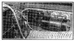
The rotary generator mounted under the dashboard.
