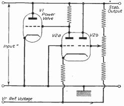
Fig. 3.—Simplified shunt regulator.
