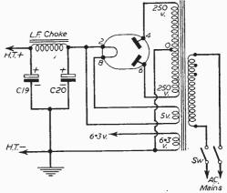
Fig. 2.—Details of a suitable power pack.
