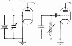
Figs. 3 and 4.—The oscillation frequency of a crystal may be shifted slightly by the above methods.
