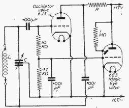
Fig. 76.4.4 method of using a "magic eve" valve to indicate a change in oscillator grid current.
