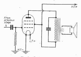
Fig. 4.—Basic output stage.
