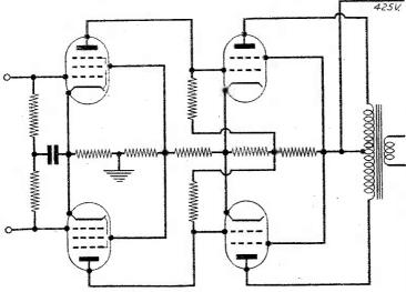
Fig. 6.-A direct-coupled amplifier.
