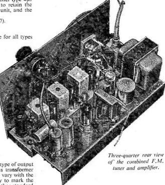
tag strip TS1 is fitted under the mains transformer, using the same nuts and bolts as are used to fix the output transformer. The other tag strip associated with VI is also fitted now, and all is ready for soldering.
