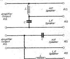
Fig. 2.—Simple systems giving attenuation of 6 db for octave layout crossover.
