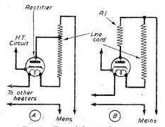
Fig. 1.—Typical line-cord circuits.
