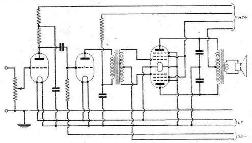
Fig. 4.—A good battery amplifier with Class B output.
