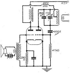
Fig. 5.—A self-excited modulated oscillator rig<sub>x</sub> using a 12AT7.
