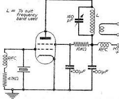
Fig. 1. — A simple crystal oscillator capable of useful output with suitable crystals for 1.8, 3.5 or 7.0 Mc/s.
