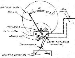
Fig. 1.—Changing a thermo-couple to milliammeter.
