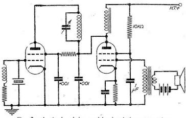
Fig. 2.—A simple choke modulated telephony transmitter,
