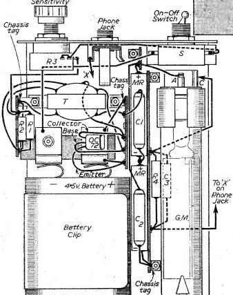
Wiring details for the counter. The collector of the OC72 is marked with a red spot.
