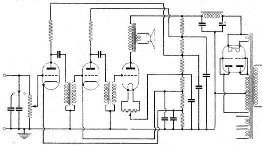
Fig. 2.—Circuit of a German amplifier.
