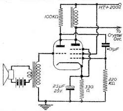
Fig. 3.—The Mullard ECL80 triode-pentode used as a two stage modulator.
