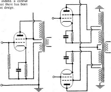
Fig. 7.-Cathode-anode output, and an American version.
