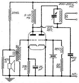
Fig. 4.—An ultra-simple QRP "one valve" phone rig using a single 12AT7.
