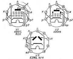
Fig. 4.—Valve holder pin connections.
