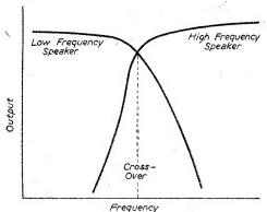
Fig. 1.—Curve showing effect of a cross-over network.
