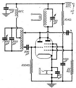
Fig. 6.—The ECL80 as an oscillator P.A. rig.
