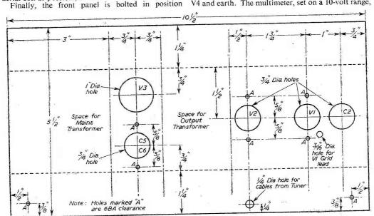
Fig. 1-Details of amplifier chassis bending and cutting.
