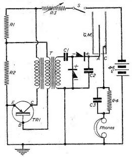
Fig. 1.—Theoretical circuit of the Geiger counter,
