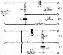
Fig. 3.—Practical systems giving constant input and good attenuation.
