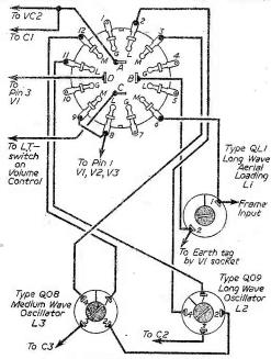
Fig. 5.—Details of the coil switching.
