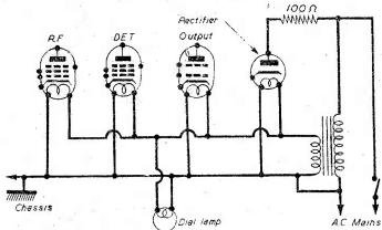
Fig. 3.—Circuit showing the use of a transformer.
