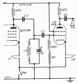
Fig. 3.—Modification to enable frequency doubling to be effected in the pentode section of the ECL80.
