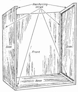
Fig. 5.—Assembly details of the case.
