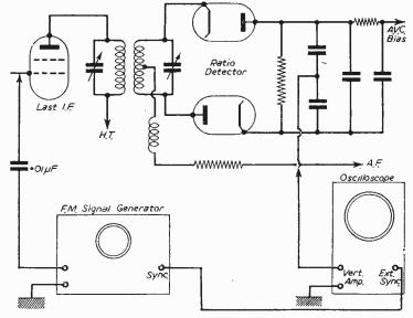
Fig. 3.—The set-up with ratio detector.
