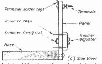
Fig. 1 (c).—Side view of panel and baseboard. The Base and Panel
