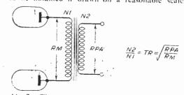
Lig. 2.—The turns ratio of the modulation translormer is calculated by the relationship shown above. RM is the required load value for the modulator valve or valves, while RPA is the effective resistance presented by the P.A. stage. N1 and N2 are the number of turns in the primary and secondary windings respectively. In practice the ratio of turns TR is all that need be known to effect a match.
