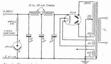
Fig. 6.-Theoretical circuit of power pack for organ and amplifier.
