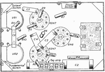
Fig. 2.—Underneath view of oscillator and " octave " chassis.
