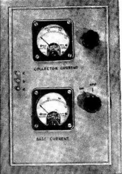
involved. The supply is a 1.5 volt dry battery, while the variable 10 K resistor is responsible for variation of the base current. A switch S is incorporated to prevent current drain from the battery when the unit is inoperative. The action of the test set is simple. The transistor having
