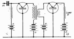
Fig. 3.—A transformer-coupled common base amplifier.
