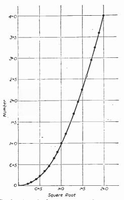
Fig. 3.—A graph of square roots produced by the "Inverse Method" of squaring a series of numbers, enables a useful square root graph, suitable for modulation ratio determination, to be drawn. The original series of numbers provides the square root values corresponding to numbers obtained by squaring the original series. As will be seen the proph was obtained by squaring a number sequence arranged in steps of 0.1.
