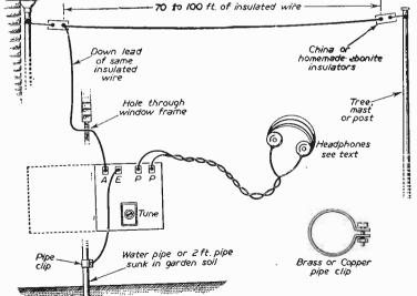
Fig. 7.-General layout for a crystal receiver.
