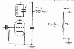
Fig. 1.—The "load impedance" of the P.A. stage for modulation purposes, is calculated as a purely ohnic resistance by Ohn's Law. In other words, the resistance corresponding to the P.A. plate current drawn at the applied plate voltage is calculated as for any other type of resistance.
