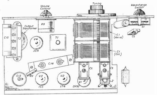
Fig. 3.—Top wiring details.
