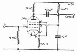
Fig. 9.- A one-valve switch.
