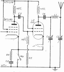
Fig. 2.—The new P.A. stage.
