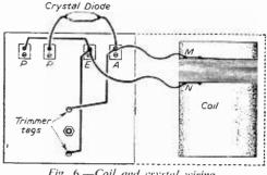
Fig. 6.-Coil and crystal wiring.
