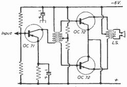
Fig. 2.—A transistorised output stage.
