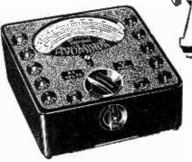
$\begin{array}{c} \mbox{MODEL I} \\ \mbox{D.C. VOLTAGE : 0 to 500 volts.} \\ \mbox{A.C. VOLTAGE : 0 to 500 volts.} \\ \mbox{D.C. CURRENT : 0 to 500 mA.} \\ \mbox{RESISTANCE : 0 to 20,000 $\mathcal{Q}$.} \\ \mbox{Total resistance of meter : 200,000 $\mathcal{Q}$.} \\ \mbox{SENSITIVITY : 400 $$\mathcal{L}$$/V.} \end{array}$
