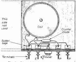
Fig. 4.—Plan of the first set, showing wiring.
