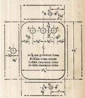
Fig. 2: Preamplifier chassis drilling details (top view).
