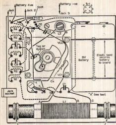
Ferrite rod secured by elastic bands round grommets and through board
