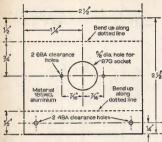
Fig. 2a: Drilling and bending details of valveholder bracket.
