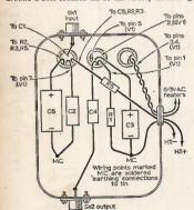
Fig. 31 Preamplifier component layout and wiring.
