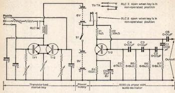
Fig. 2: Diagram of electronic key and phase-shift audio oscillator.
