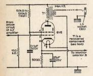
Fig. 4: Output stage, showing monitor point.
