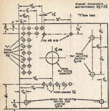
Fig. 3: Drilling details for the banel.
