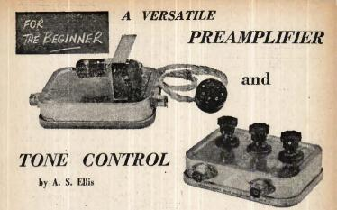
In the field of audio, need is often felt for an unspecialised preamplifier capable of being used with a wide variety of equipment for various purposes not necessarily forming a permanent part of any of these pieces of equipment. The particular preamplifier to be described was originally built to give greater sensitivity to a somewhat insensitive "gram" amplifier unit has, however, since then been used with enormous success in a number of other applications.
