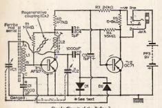
Fig. 1. Circuit of the Reflex 2.
