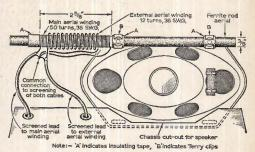
Fig. 5: (above) Aerial winding and mounting details
