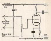
Fig. 2: The arrangement of a valve amplifier input stage for connection of the preamp. R has a value to regulate the amplifier h.t. to 250V for the preamp. C=8µF 350V.
