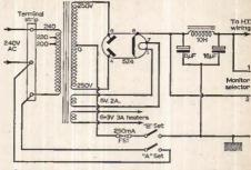
Fig. 5: Power supply circuit, showing monitor points and h.t. control.
