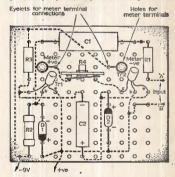
eyclets and the terminals when the terminal nuts are tightly screwed down. In this way, therefore, the module is secured to the meter movement.
