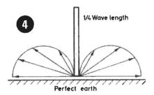
The Marconi aerial radiates equally well in all directions round the aerial, i.e. it is omnidirectional.
