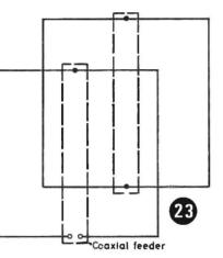
Mount each element on small insulators on vertical pieces of wood, shown dotted. Use another piece of wood as a boom to fix the elements 450mm (18in) apart.
