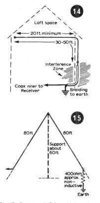
then the lower part of the aerial can be a length of coaxial cable with the outer screen connected to the receiver chassis or earth, Fig. 14.
