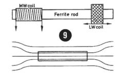
virtually nothing off the ends. Such aerials are used in domestic MW and LW receivers but the fact that they are so directional is often overlooked. It is highly desirable that the set be turned round for maximum pick-up of weaker stations. Ideally the rod should be rotatable independently of the receiver. Ferrite rod aerials for the SW bands are not very common in this country.
