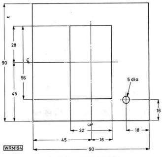
Fig. 3: Front panel details
