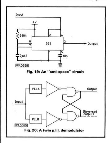
sistor of Fig. 18. Such a circuit, based on a 555 timer, is shown in Fig. 19. This circuit (first suggested by VE4CM) passes normal RTTY signals, but if a space longer than about 300ms appears at the input the output will switch to mark and prevent further "clattering".
