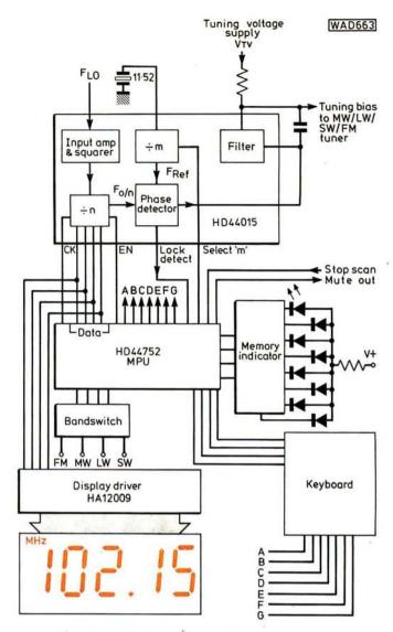
Fig. 2: Block diagram of the Hitachi HD44752 frequency synthesis system
