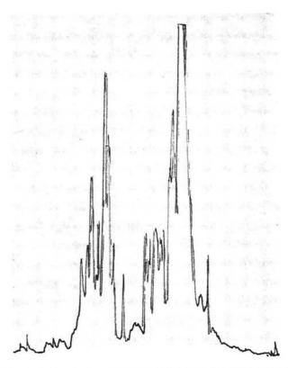
Fig. 1: A 4-minute solar burst, recorded by the author at 136MHz around midday on July 20
