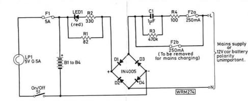
Fig. 1: The circuit diagram of the rechargeable handlamp
