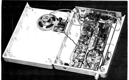
The two p.c.b.s forming the Wood & Douglas 70cm single channel transceiver. The receiver board is the top one. Although both boards are tightly packed with components, and double-sided, no problems were found during assembly
