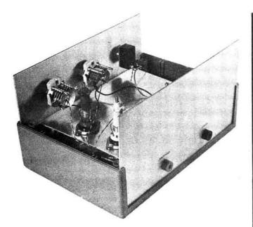
A view of the receiver with the top of the Verobox removed showing the location of the chassis subassembly within the case
