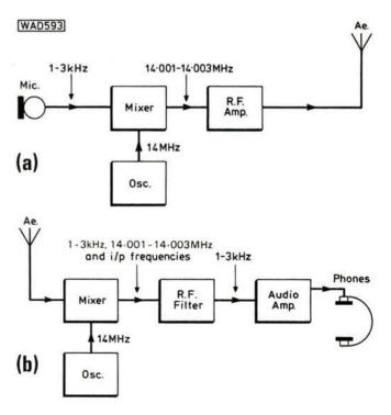
Fig. 1: Block diagrams of a simple u.s.b. transmitter (a) and receiver (b)
