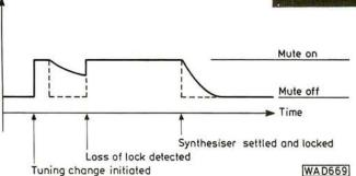
Fig. 9: Muting output after processing. The dotted line shows the actual MPU output pulses before stretching
