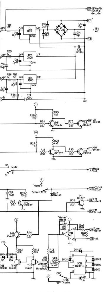
Fig. 3: Complete circuit diagram of the synthesiser unit. The boxed numbers indicate off-board connections to tuner and stereo decoder modules and mains transformer. Output pins on IC3 go directly to the 7LT02 fluorescent display. Layouts for the two p.c.b.s will be given later in the series
