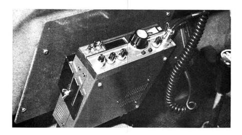
five, so that non-standard frequency offsets can be programmed if required. Two forms of scanning are provided: Memory scanning, in which the contents of either memory bank are scanned, and Band scanning which looks at the spectrum between the frequency programmed into memory channel A5 and that in channel B5.
