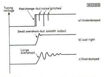
Fig. 6: Effect of filter time-constant on tuning action
