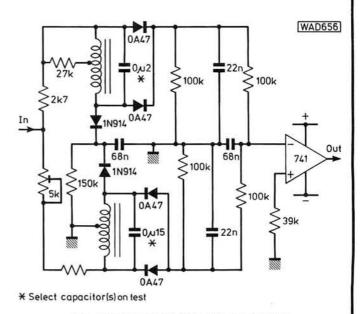
Fig. 15: A passive filter demodulator
