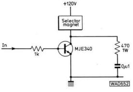
Fig. 12: A TTL to single current interface
