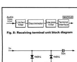
Fig. 9: Terminal unit input limiting
