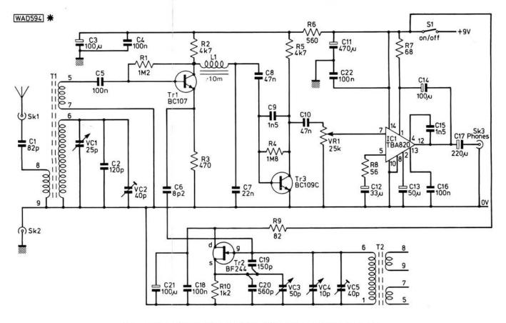
Fig. 2: The circuit diagram of the Direct Conversion Receiver
