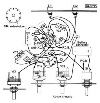
Fig. 4: Chassis wiring diagram. Note that VC1 (ANT. TRIM) and VR1 are both mounted below the chassis. Do not forget to check that the negative battery connection is properly made to both the chassis and the printed circuit board
