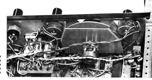
A close-up of board 1 and of the mounting for VR14, which had an integral 10:1 slow motion drive on the prototype unit. A separate s.m.d. with dial drive facilities can be used instead
