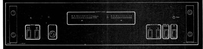
\* Two toroidal PSUs of 250VA rating \* over 140W into 4 ohms \* Speaker relay with switch-on delay \* Peak output bargraph \* Exceptionally well documented (instruction manual £2.50 available separately), repeatably low distortion (-65dBmin), very rugged.
