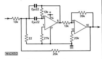
Fig. 10: Active band-pass filter
