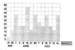
Fig. 3: Rounded numbers of East European broadcast stations heard during a SpE event between 65-73MHz
