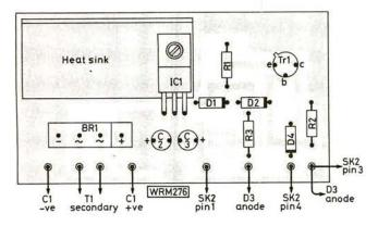
Fig. 2 (top): The copper track pattern of the p.c.b. shown full size
