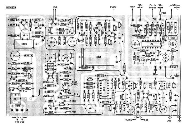
capacity, adjust T9 for maximum output at 28MHz. Now switch S5 to 29–30MHz and set VC1 and VC2 to one third of maximum capacity, adjusting VC5 for maximum output at 30MHz. Repeat these operations for maximum output at each frequency.
