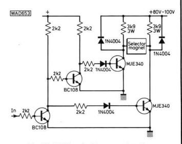
Fig. 13: A TTL to double current interface
