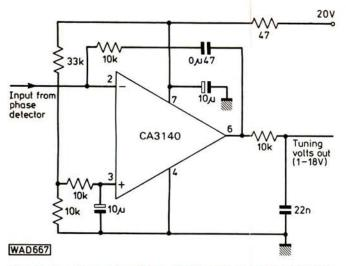
Fig. 7: An alternative form of filter-integrator suitable for driving high-voltage tuning lines
