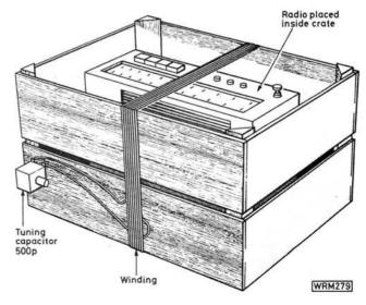
Fig. 1: The Tiny Loop, as designed by Dilip Kapur
