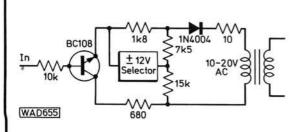
Fig. 14: A TTL to ±12V interface
