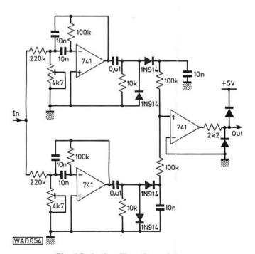
Fig. 16: Active filter demodulator
