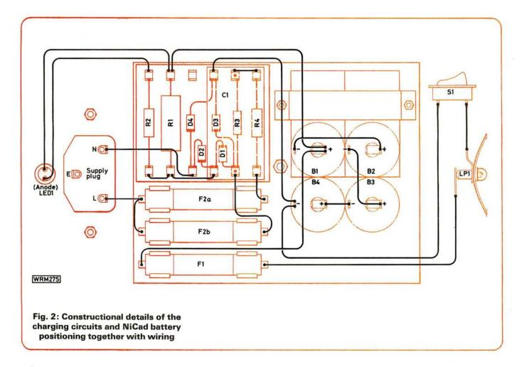
circuited the bridge would be required to support the full mains voltage. For this reason it is best to use at least 600V diodes, such as 1N4005, as their extra cost is negligible. The use of high-voltage diodes also ensures that the bridge has an extremely low reverse-leakage current which prevents the NiCad battery being significantly discharged through the diodes over a long period of storage.
