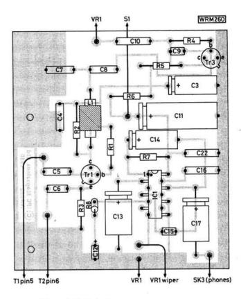
Fig. 3: The foil pattern and component layout (full size)
