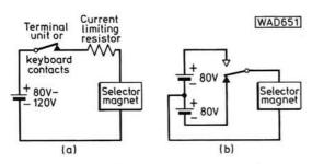
Fig. 11: (a) Single current signalling. (b) Polar or double current signalling
