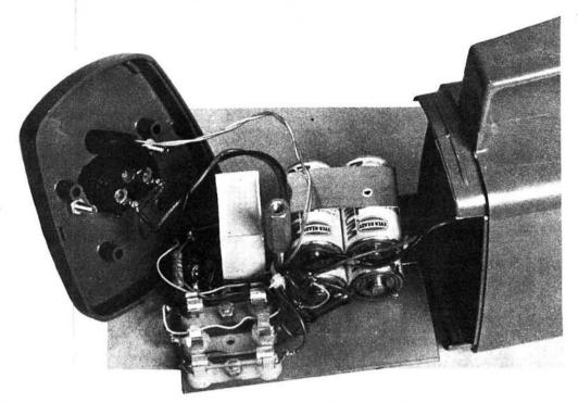
If there is no likelihood of charging from a car battery then fuse holder 2b need not be incorporated and the rating of R1 may be reduced to 1W. Similarly, if a car battery is to be the sole source of charge, fuse holder 2a, R4, C1 and R3 need not be provided.
