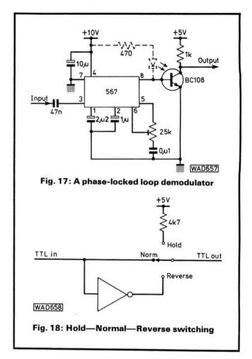
power supply, this circuit provides a complete RTTY demodulator. The centre frequency of the p.l.l. is set by the  $25k\Omega$  preset potentiometer, which should be of the multiturn type.
