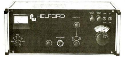
A 120W p.e.p. rig designed around a new transceiver p.c.b. from Plessey which is surely destined to replace the famous G3ZVC board. The initial design is for 80 and 20m, and a further module will be ready shortly to add 40, 15 and 10m too. If you don't need so much power just omit the p.a.—the driver will give up to 25W
