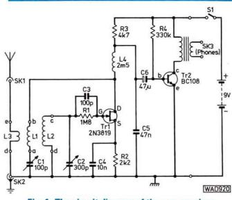
Fig. 1: The circuit diagram of the s.w. receiver
