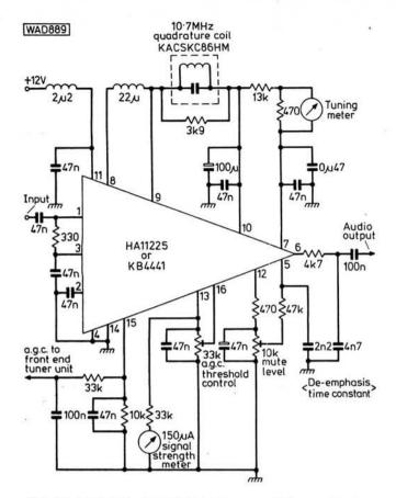
Fig. 2: A simple circuit for the use of these devices using a single-tuned KACSKC86HM quadrature coil
