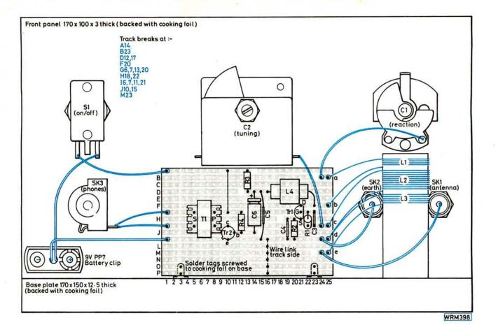
the variable capacitors' fixed vanes and antenna and earth sockets. The switch, output socket and battery connector leads may now be wired to the Veroboard. The wiring is checked, battery and headphones connected and the power switched on. If a loud hum emanates from the headphones when a finger is placed on C3 the circuit is probably functioning correctly.
