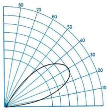
$\lambda/2$  antenna, gain 2dB radiation angle 35°
