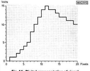
Fig. 11: Digital representation of signal
