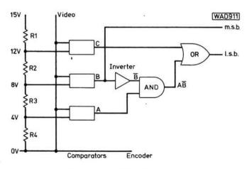
Fig. 12: 2-Bit A-D Converter
