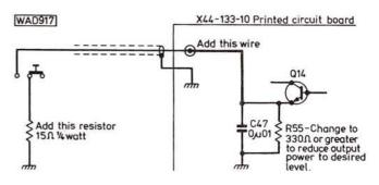
If you decide that you would like an even lower output, simply increase the value of the Q14 emitter resistor, but keep in mind that the value of the emitter resistor and the sub-tone switch resistor when connected in parallel must equal  $10\Omega$  if you want to maintain full output power when the switch is open.
