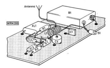
Fig. 12: Component layout details of the oscillator
