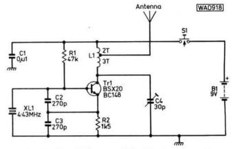
Fig. 11: Circuit diagram of the i.f. alignment aid
