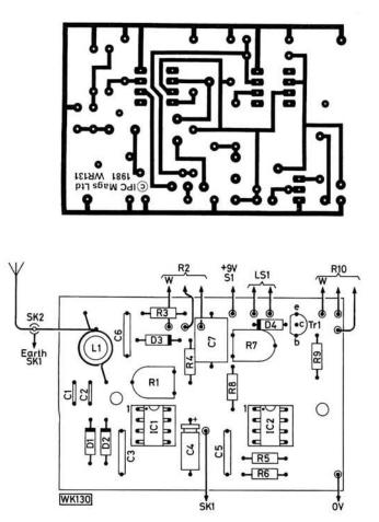
Fig. 2: Track pattern and component layout of the meter
