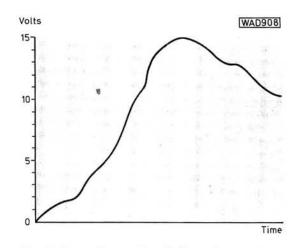
Fig. 9: An analogue signal of one line of video
