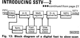
Fig. 13: Block diagram of a digital fast to slow-scan line converter
