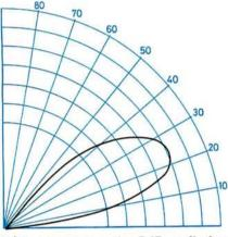
5/8λ antenna, gain 3dB radiation angle 30°
