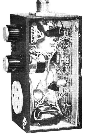
trying to tune in a weak field with the sensitivity turned up. Note that R2 sets the d.c. output voltage of IC1 for a given r.f. field.
