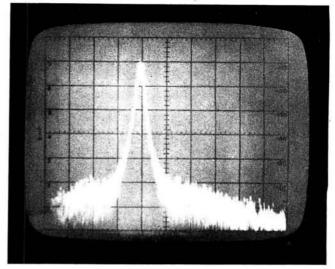
Fig. 45: This photograph shows a single tone at 18W output. The difference between Figs. 43 and 45, the carrier suppression, may be seen to be approximately
