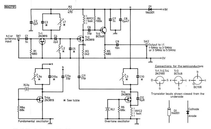
Fig. 2: Circuit diagram of the h.f. converter
