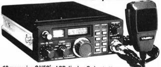
10 memories, 2 VFO's, LCD display, C size battery, easy car mounting tray, 2.5 watts out.
