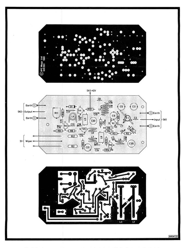
Fig. 2: Track patterns and component layout, both shown full size. Component leads to be soldered on both sides of the p.c.b. are indicated by dots on the component layout drawing
