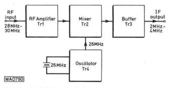
Fig. 1: Block diagram of the h.f. converter. Frequencies shown for 10m amateur reception
