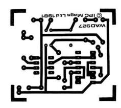
Fig. 2: The track pattern of the p.c.b., shown full size
