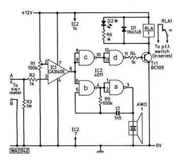
Fig. 1: The circuit diagram of the s.w.r. warning alarm
