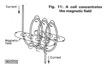
By adding little arrows to the letters "N" and "S", to indicate the direction of the current, you can then easily remember which direction causes a south or north pole.
