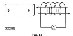
Dynamos and generators operate by electromagnetic induction, converting mechanical energy into electrical energy.
