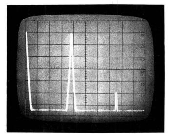
Fig. 44: The fundamental frequency plus the second harmonic at 80m. This may be seen to be approximately 50dB down on the wanted signal. The noise floor at about 65dB down is the only other signal present; all other spurii are therefore >60dB down
