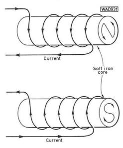
Fig. 12: Field direction in a solenoid
