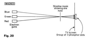
which glows blue when energised by an electron beam, whilst the other two glow green and red respectively.
