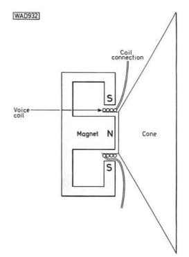
Fig. 13: Loudspeakers use the effects of electromagnets to produce their sound
