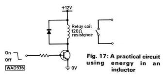
When the transistor is switched off, the counter e.m.f. in the coil could reach a value of several hundred volts positive at the transistor collector and damage the transistor. To prevent this happening a "catching" diode is connected across the coil, as shown, and conducts when the counter e.m.f. occurs at switch-off. The counter e.m.f. then drives a current through the coil and the energy is dissipated in its resistance.
