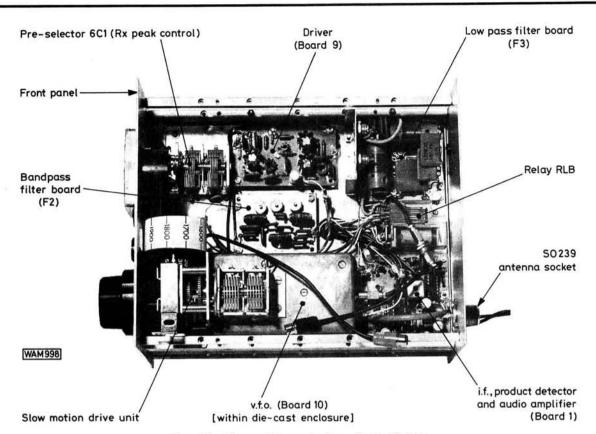
Fig. 41: General layout plan view of the transceiver upper side
