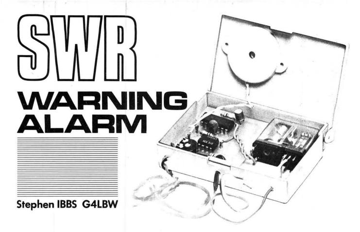
One of the main worries of a radio operator is of transmitting either without an antenna or with a faulty antenna connection, resulting in a high s.w.r. and, often, a useless p.a. stage. This design provides an alarm in such circumstances, with the option of automatically switching the transmitter off.
