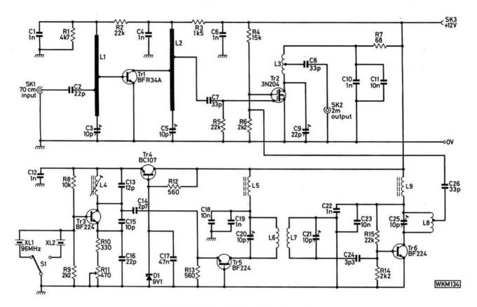
Fig. 1: Circuit diagram of the converter
