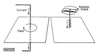
Fig. 10: The direction of a magnetic field shown by the corkscrew rule
