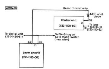
There are no external changes to the set as the mode switch (S3) is used to initiate the reverse repeater function by using the FM-B position to activate the correct shifts on both 2m and 70cm, -600kHz and +1.6MHz respectively. The FM-A position provides reverse repeater operation when the "SHIFT" button is depressed. The alternative shifts that were available are disabled by the mod to the mode switch.
