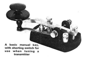
Because the back contacts will open before the front contacts close, and will not close again until after the front contacts have opened, there is a time overlap which can, for example, be used to protect an associated receiver by removing its antenna and/or applying a desensitising bias whenever the transmitter is radiating. In the modern transceiver, such functions are usually carried out by an internal transmit/receive relay, or electronic switching.
