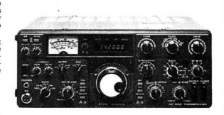
A recent addition to the Trio HF range, and proving amazingly popular is the new TS530S. Designed as a "little brother" to the TS830S, the TS530 uses the same PLL system, same RF boards, same readout system and many other features of the 830 but without the variable bandwidth facility. You do, of course, have the famous Trio I.F. shift system for dodging the QRM.
