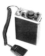
For those of you who enthuse over portable SSB operation on the hills and mountains of the UK, or wish to chat to the local lads whilst seated by your fireside, then the Mizuho SB2X 2 metre SSB portable is the rig for you. One watt output on the SSB frequencies 144.000 to 144.600 and the ability to listen to the beacon frequencies from 144.800 to 145.000 (also transmit)
