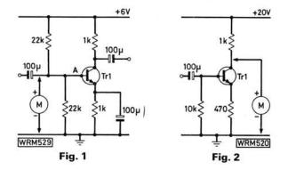
close to the quoted figure, yet in certain circumstances a reading of +1.3V could be **exactly correct**. Take the circuit in Fig. 2. Suppose the meter reads +19.5V. Is this correct? Since the transistor is non-conducting it seems to be near enough, yet if the supply is indeed +20V, this reading could indicate a faulty component! We shall return to these problems in a later article.
