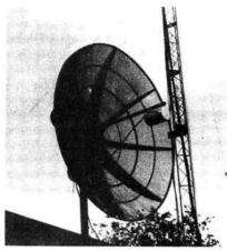
Fig. 6: 2.5m dish for 1296MHz
