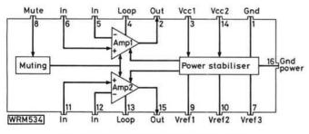
Fig. 1: Block diagram of the KB4433
