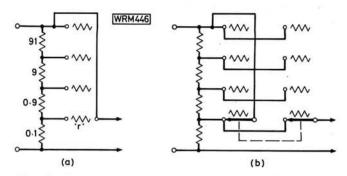
Fig. 2: Overcoming problems due to switch contact resistance on the current ranges
