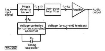
Fig. 1: The basic phase-locked-loop in block form
