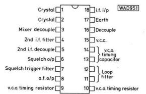
Fig. 2: Connections of the SL6600C
