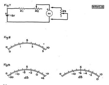
Now connect variable resistor R3 across the meter terminals and adjust it until the meter reading drops to half-scale. Use a  $2.5k\Omega$  potentiometer for R3.
