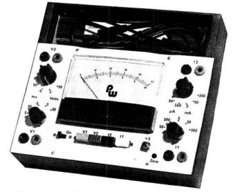
Each t.p. would have to be completely isolated by the 4way selector switch, so that they could be scattered anywhere around a circuit, and be at different potentials.
