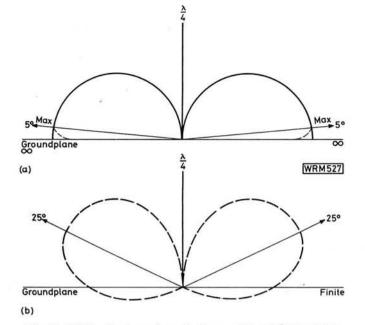
Fig. 3: (a) Vertical angle radiation pattern of a quarterwave vertical antenna over a perfectly conducting ground-plane of infinite dimension. (b) When the ground-plane is of some infinite dimension, e.g. one wavelength and consists of a number of radials, the vertical angle of maximum radiation is tilted to about 25 degrees
