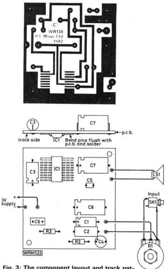
Fig. 3: The component layout and track pattern shown full size
