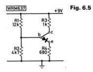
base-collector is open-circuit. To verify this we could unsolder the transistor and test it, but we would probably find it checked out all right and we would have to think
