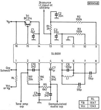
Fig. 3: A SL6691 circuit for demodulating an f.m. signal and providing a paging output if required
