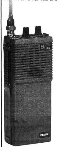
10W p.a. The rig comes supplied with a "rubber duck" antenna but its coverage can be greatly improved by using a 430MHz colinear—the antenna socket being a BNC type.
