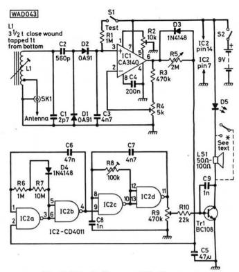
Fig. 3: Circuit diagram of the time-out alarm
