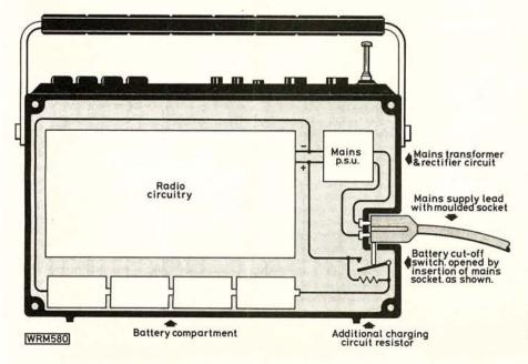
Fig. 1: Schematic layout of an average mains/battery portable radio showing the modification required to provide charging current when using a NiCad battery pack.
