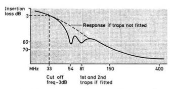
Fig. 3(a): Typical frequency response of low-pass filter (not to scale). The series tuned traps (if fitted) will normally be tuned to the second and/or third harmonics of the 27 to 30MHz band. The basic circuit is as shown
