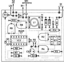
Fig. 2: Track pattern and component layout for the p.c.b. shown full size
