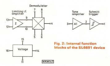
pin 12 (R3) and from pin 9 through the  $2k\Omega/33nF$  filter network to pin 13 (R2) are essential, since they provide the feedback necessary to maintain the correct operating point of the limiting i.f. amplifier. Pin 12 is decoupled to ground, so that the feedback is effective only at zero frequency, i.e. for d.c. currents. Similarly capacitor C2 decouples the junction of resistors R1 and R2 to ground.
