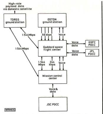
Fig. 4: Flow diagram of ground communications
