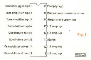
The SL6691 is encapsulated in a 16-pin dual-in-line
