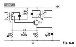
No. 2: Estimate the correct e, b and c potentials of the transistor in the i.f. amplifier circuit of Fig. 6.8.
