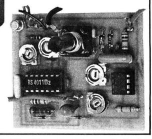
Switch S1 provides a convenient means of testing that the unit is working and is also used in the initial adjustment procedure. When closed, a slight positive potential is applied to pin 3 of the CA 3140, causing the output to rise to maximum, and starting the pulse train.
