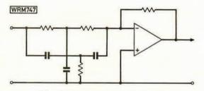
Fig. 1: The basic bridge circuit
