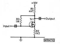
If the voltages are incorrect, you may suspect the IGFET itself of being faulty and wish to remove it for testing by ohmmeter. **DON'T!** Insulated gate devices **must not** be tested by ohmmeter—the test itself would probably destroy them. This is because the g-s capacitance is extremely small and its breakdown voltage is limited.
