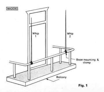
Two mobile type 14MHz (20m) whip antennas should be clamped to the iron railings which surround the balcony of many flats, as shown in Fig. 1. Then, run two equal lengths of 50 ohm coaxial cable to a metallic junction box, terminated into a pair of UHF SO239 sockets, SK1 and SK2 of Fig. 3. What we are now going to do is to feed these two whip antennas out of phase to obtain an "end fire" directional beam effect.
