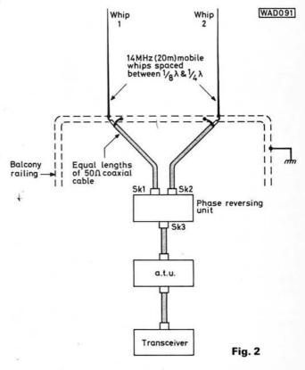
Try and obtain as good an earth as possible, but you will find that good performance should be obtained just using the iron railings alone. Different lengths of coaxial cable can be tried between S1 (b) and SK3 — the longer you make it, the greater is the degree of phase shift. Do
