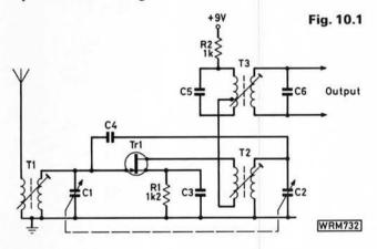
No. 1: Given that the source potential was +2V, and oscillations and signals were suppressed, you were asked to estimate the gate and drain potentials with respect to earth.
