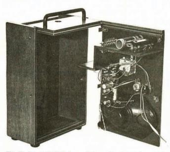
Fig. 5: An exploded view of the author's receiver and its wooden case. The wires disappearing to the right are connected to the 9V battery
