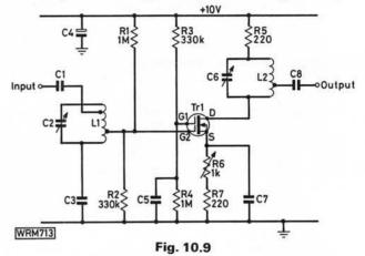
This month's problem is based on the circuit of Fig. 10.9, an r.f. amplifier with gain control (R6). Under nosignal conditions, source potential is measured as  $+3\cdot1V$ (R6 at minimum resistance) and +4V (R6 at maximum resistance). Estimate the potentials at g1, g2 and d for both these extreme settings of R6.
