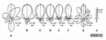
Fig. 2.3: Radiation patterns of a nominal 400-450MHz six turn helical antenna across the range 275-560MHz
