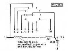
Fig. 3: Circuit of a.t.u., matching wire antenna to receiver on any h.f. band. Cardboard centre of toilet roll makes ideal coil former. Prick small holes at one end to anchor wire, wind on two turns, scrape wire clean and twist small loop. Leave 3mm space, wind on two more turns, make another loop, space, three turns, make loop, and so on. The coil is mounted directly on capacitor and switch. Use insulating panel to isolate capacitor or mount on insulating pillars on aluminium panel
