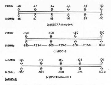
Fig. 2.1: The relationship between uplink and downlink bands for OSCAR 8 and RS3-8
