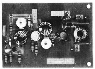
A completed transmit board is shown above. The mechanical construction is shown at the top of the next column with a completed v.f.o. below
