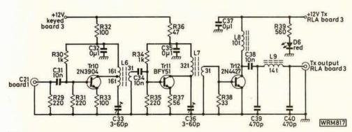
Fig. 3.1: Circuit diagram of the transmit section of the PW 'Severn'
