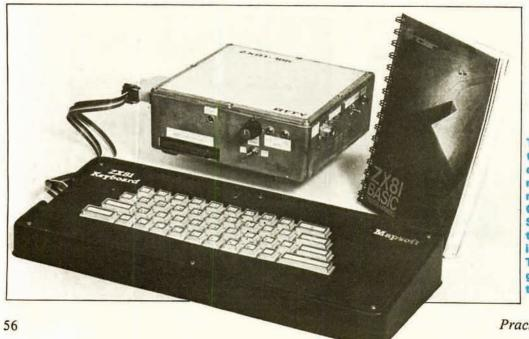
The re-housed ZX81 with the Maplin keyboard. The diecast box houses the mains power supply, mains filter, ZX81, Ground Control 16K RAM board, Scarab interface board together with the various input and output sockets. The Maplin keyboard is a great improvement over the original ZX81 pressuresensitive one
