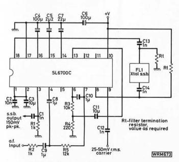
Fig. 9: A very simple s.s.b. generator
