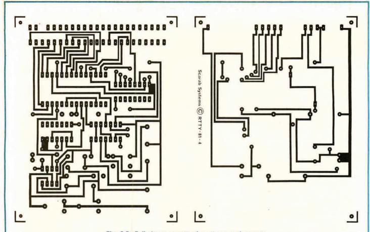
Fig. 2.2: Full-size copper track patterns and component placement for the Scarab Systems interface board
