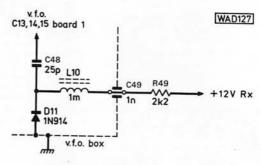
Fig. 3.6: The small offset circuit
