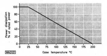
Fig. 1.1: Typical power derating curve for silicon semiconductors
