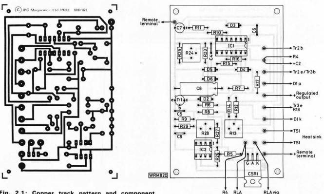
Fig. 2.1: Copper track pattern and component placement shown full size
