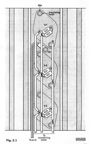
the case. The heatsink extrusions must not cover the slot in the back of the case but are mounted just above the slot. Air is then forced out of the case by the fan and up over the heatsink fins.
