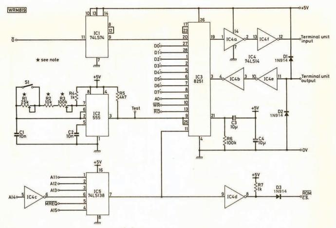
Fig. 2.1: Circuit diagram of the Scarab Systems interface. Resistor R2 can be replaced with a variable resistor to give a fine baud rate control if required.
