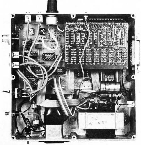
The complete 16K ZX81 fitted into a large diecast box. The Scarab Systems RTTY interface board is fitted at the top left of the box while the Ground Control 16K RAM board, taken out of its plastics case is mounted directly above the ZX81 board in the top right corner. The mains power supply is in the bottom right of the box with the mains filtered plug centre bottom
