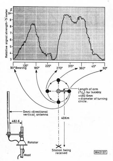
Fig. 6.4: Showing the pen chart recording of v.h.f. signal variation due to phase effects, also the rotation of the v.h.f. vertical antenna on a radius of λ/4
