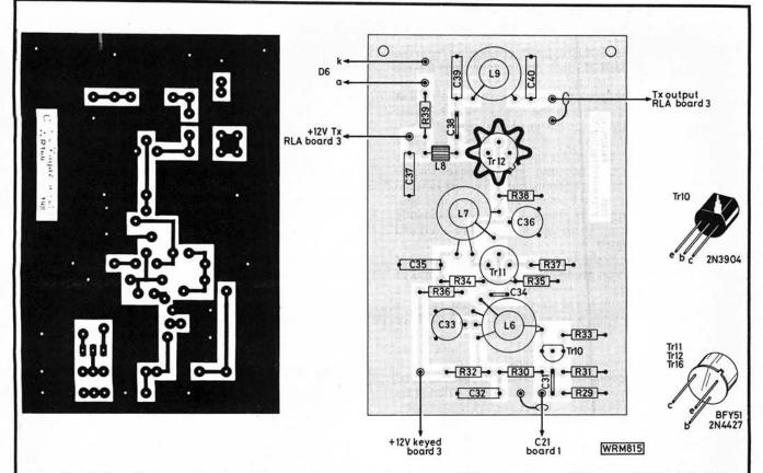
Fig. 3.4: (Above) copper track pattern and component placement for the transmit board shown full size. Fig. 3.5: (Below) the copper track pattern and component placement for the changeover and sidetone board shown full size. The photograph shows a completed sidetone and changeover board
