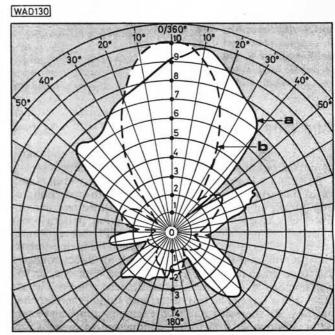
Fig. 6.2: The distortion of the radiation pattern due to the four silos
