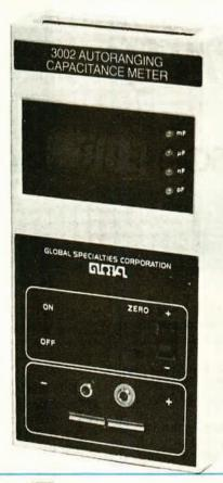
and the instrument automatically selects the most appropriate of the eight ranges. The basic accuracy is claimed to be 0.2 per cent of reading  $\pm$  1 count up to  $199.9\mu F$  and 1 per cent of reading  $\pm$ 1 count up to 19.99m F with a resolution of 0.05 per cent of full scale on all ranges and 1pF on the lowest range.
