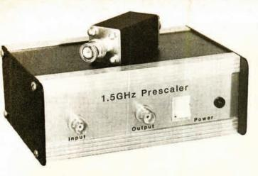
This article describes the construction and use of a prescaler module enabling frequencies in excess of 1.5GHz to be measured with a frequency counter covering 500MHz. It may be constructed as a complete, self-powered unit, or as an add-on accessory, powered from an existing supply source.
