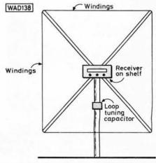
Fig. 1. Receiver attached to loop
