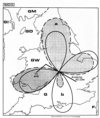
Fig. 6.5: Distortion of the radiation pattern from a long wire antenna operated on the h.f. bands
