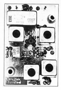
herent with diode switching. This is followed by a BF981 in an input noise-matched, output conjugately matched configuration for a very low noise figure and optimum dynamic performance. After an on-board attenuator
