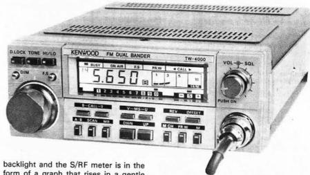
form of a graph that rises in a gentle curve as the signal strength increases.
