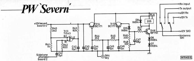
Fig. 3.3: Circuit diagram of the change-over and sidetone generator
