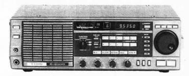
and later in the year for the **R 2000** a 118 to 174 MHz internal vhf converter.
