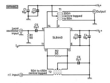
Fig. 4: A high performance balanced circuit
