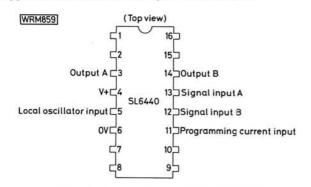
Fig. 1: Connections of the SL6440
