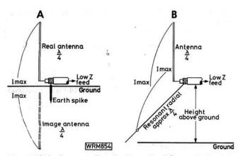
Fig. 8.2(A): Current distribution of a  $\lambda/4$  vertical with base at ground level and (B) in conjunction with resonant horizontal radial
