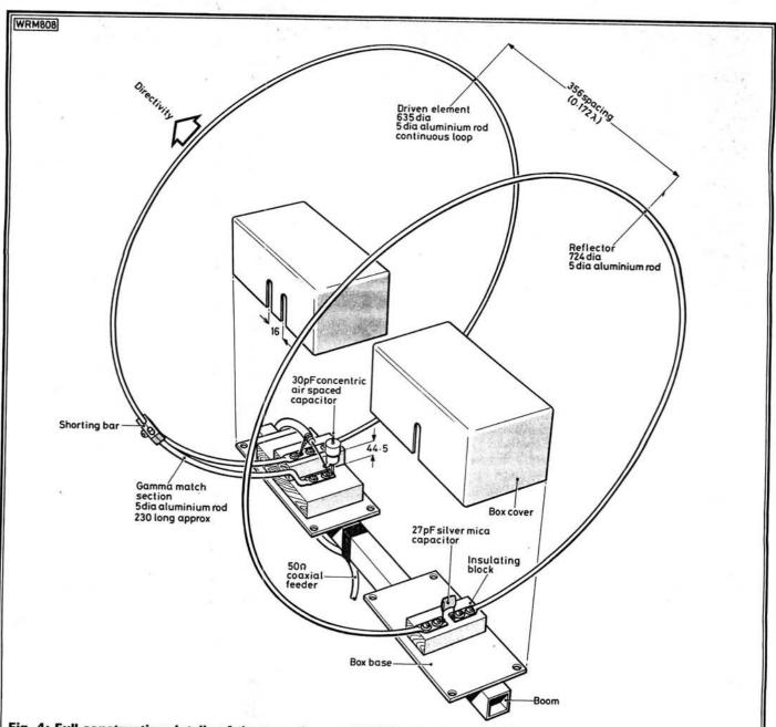
Fig. 4: Full construction details of the two-element 144MHz ring beam antenna. The boom may be connected to the supporting mast by means of a bracket located between the elements as shown in the photograph on page 26. As drawn, the antenna is horizontally polarised; rotating the boom and element assembly through 90 degrees will provide vertical polarisation
