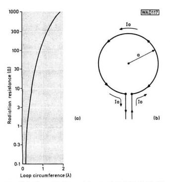
Fig. 2(a): The radiation resistance of circular loops up to  $2\lambda$  diameter. The Rr of a  $\lambda/\pi$  diameter loop is approximately 150 $\Omega$  (b) Direction of current (in-phase) around a circular loop  $\lambda/\pi$  diameter. Points of maximum current are designated as lo
