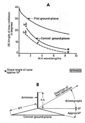
Fig. 8.6(A): Angle of maximum radiation obtainable using flat disc ground-planes of various radii and (B) angle of maximum radiation using conical groundplanes
