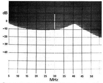
Spectrum analyser plots of the filter. Above C1 = C2 = C3 = 10 pF. Below C1 = C2 = 40 pF, C3 = 10 pF. By varying C1 and C2 it is possible to alter the characteristics
