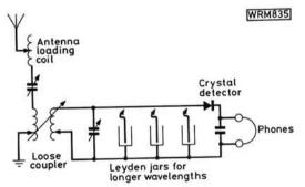
Fig. 5: The circuit of a typical crystal receiver
