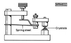
Fig. 8: A Perikon two-crystal detector Practical Wireless, September 1983
