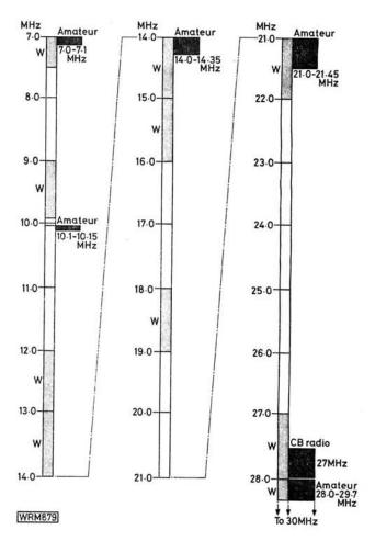
Fig. 2.5: Usage of the frequency band 7–30MHz by the Russian OTHR
