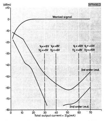
Fig. 2: Variation of 2nd and 3rd order intermodulation levels with the total output current (Signal frequency 30MHz) Practical Wireless, September 1983
