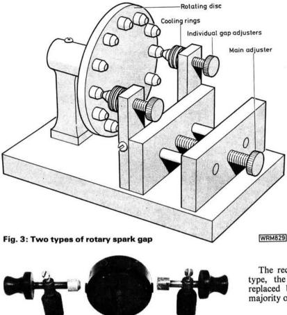
The voltage supply for the spark gap was normally provided by an induction coil with a make and break set of contacts fed from a suitable battery (the same principle as now used for coil ignition in petrol engines). Almost any form of regular switching of the d.c. supply was applied to the induction coil primary.
