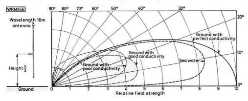
Fig. 8.4: Vertical angle radiation from vertical  $\lambda/2$  with centre point  $\lambda/3$  above ground showing effects of ground conductivity
