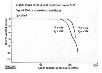
Fig. 5: Frequency performance of the SL6440
