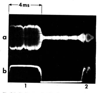
Fig. 2.1: Oscillogram showing the expanded "Woodpecker" pulse (a) unrectified (b) rectified
