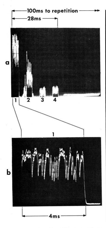
Fig. 2.6: Four pulse modulated "Woodpecker" signals
