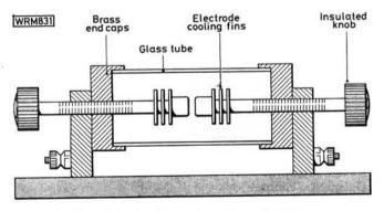
Fig. 4: A simple enclosed spark gap
