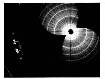
Fig. 5: Radiation pattern of a single loop of diameter  $\lambda$  taken from a 941.9MHz model
