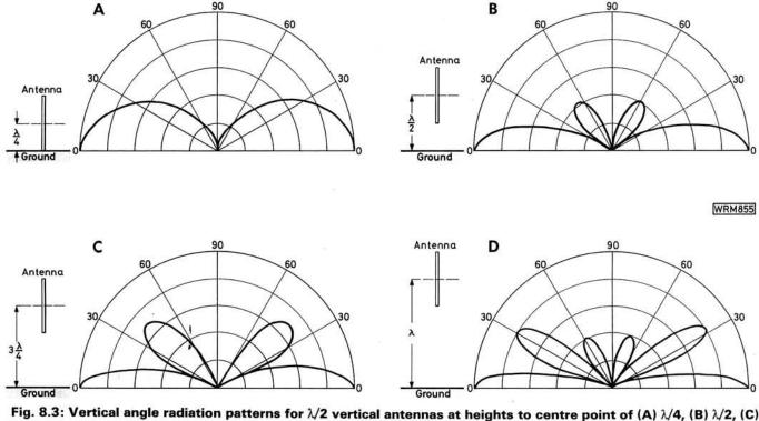
Fig. 8.3: Vertical angle radiation patterns for  $\lambda/2$  vertical antennas at heights to centre point of (A)  $\lambda/4$ , (B)  $3\lambda/4$ , (D)  $\lambda$
