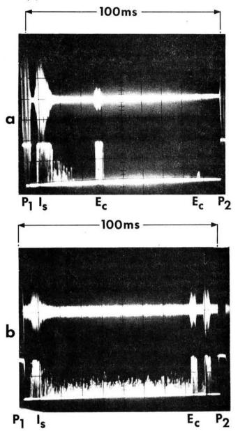
Fig. 2.3: Single pulse signals (a) unrectified (b) rectified/amplified
