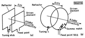
Fig. 3(a): Configuration of a two-element quad antenna for optimum gain/smallest amplitude rear and side lobes (b) Configuration of two-element circular loop antenna for optimum gain and no significant rear/side lobe amplitudes
