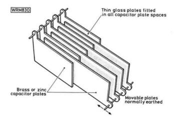
Fig. 2: An early form of adjustable capacitor
