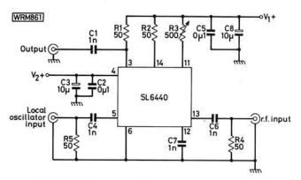
Fig. 3: A simple single-ended mixer circuit
