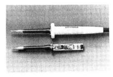
off outside a temperature band centred on the set value. Within this proportional band, power is supplied in regular pulses of equal interval but of a length which varies according to the difference between "actual" and "set" temperatures. This feature provides extremely close control, with no swing or overshoot. An internal neon indicator glows through the translucent handle when the element is energised.
