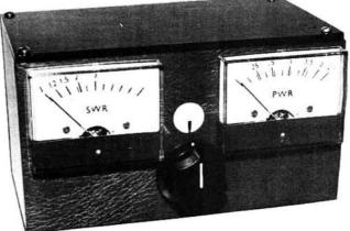
reflected readings are obtained simultaneously on the two meters M1 and M2, and the bridge is matched and balanced at the required load impedance by C1 and C2. Brief details are given in Fig. 5 of an alternative, less expensive, single meter version.
