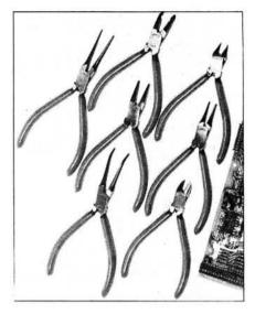
conditions, the new Draper pliers are all manufactured in induction hardened chrome vanadium steel with blue pvc coated handles. A lap joint combined with precision machined jaws ensures accurate register at the tip of the nose of the pliers, and the handles are spring loaded to minimise user fatigue.
