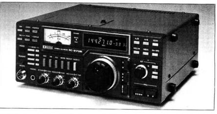
Optional extras include; speech synthesiser announcing displayed frequency; 22 channel memory extension—with scan facilities; 10Hz tuning facility and internal "chopper"
