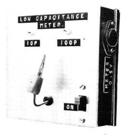
The ratio of capacitance between the maximum test capacitance (10pF or 100pF) to that of C1 or C2 has been made high in order to ensure that the signal voltage across the lower capacitor varies in a substantially linear fashion. This ratio will be seen to be about 10:1.
