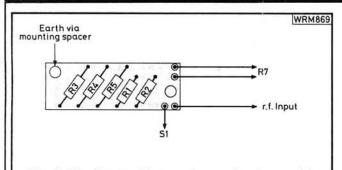
Fig. 6: The fixed resistance dummy load assembly
