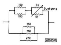
Fig. 2: A variable Q.R.P load
