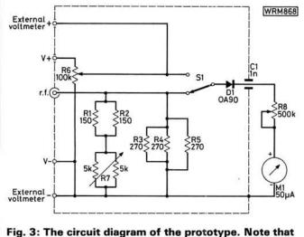
C1 is now a feed-through capacitor providing r.f. isolation for M1 as an additional function Another useful variation is to make R2 adjustable. This enables instant achievement of meter f.s.d. if different power ranges are to be used, simply by substituting a  $500k\Omega$  linear potentiometer for R2.
