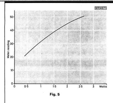
since it was decided to make up tables and graphs for various power ranges to be read off from the existing 0-50 scale (Fig. 5). Three pairs of connecting leads were made up—for the calibrating power supply; the external voltmeter; and for measuring the load resistance via the r.f. input socket. The final terminations of these leads depend on the meters and power supply to be used.
