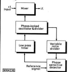
Fig. 5: The type of circuit used in many modern receivers using full frequency synthesis with the tuning at 10 or 100Hz intervals, suitable for frequencies into the u.h.f. range
