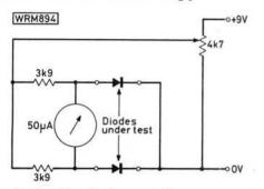
Fig. 4: A simple diode matching circuit. The two resistors should be matched with an ohmmeter. As the voltage is increased by rotating the potentiometer the meter should not deflect more than 1μA from its nocurrent setting. It may be necessary to test several diodes before a matched pair is obtained
