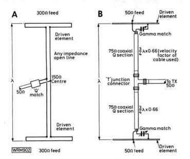
Fig. 9.2: (A) Two stacked folded dipoles fed in-phase via an open line (see text). (B) Two gamma matched dipoles with 50 $\Omega$  feed impedance, phased by a pair of 75 $\Omega$  "Q" sections of coaxial cable
