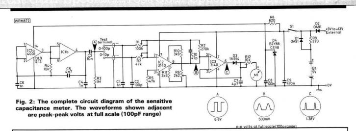
acts like a Class C amplifier in that only parts of the negative half-cycles at pin 2 are amplified, these giving a positive-going output at pin 6. A combination of a.c. and d.c. feedback ensures a linear input/output voltage relationship. The MOSFET op. amp. was chosen in preference to the usual 741 as it will continue to operate on these negative half-cycles, when its input voltage falls below earth potential. This avoids the complication of double or split supplies.
