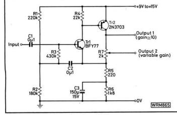
This circuit was designed primarily for a gain of ten.
