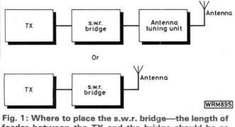
feeder between the TX and the bridge should be as short as possible
