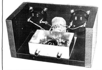
line it will show the s.w.r. presented by the antenna system to the bridge without any immediate adjustment being possible. By checking the s.w.r. at different frequencies across a band it will, however, show the effective bandwidth of the system and indicate whether alterations to the dimensions of the antenna are necessary to bring it to resonance at a higher or lower frequency.
