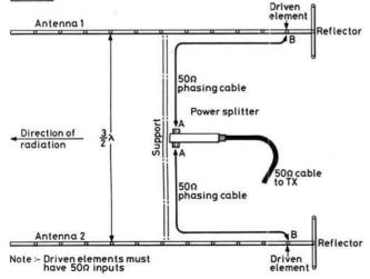
Fig. 9.3: A pair of beam antennas stacked  $3\lambda/2$  apart phased and fed via a two-way power splitter and phasing lines an equal number of  $\lambda/2$  multiples long
