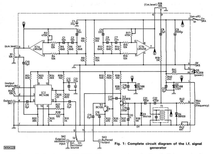
A 12 volt stabilised supply is obtained for R44 by R40 and D2 and the range of frequency shift that R44 provides can be varied by R43. The method of setting up R43 is given later.
