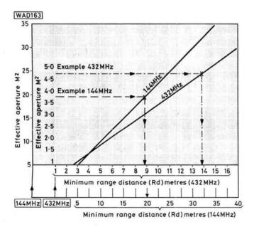
Fig. 10.5: The graph shows the minimum range requirement (Rd<sub>min</sub>) for various effective apertures for both 144MHz and 432MHz antennas
