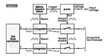
Fig. 2: Block diagram showing the operation of the d.r.i. circuit
