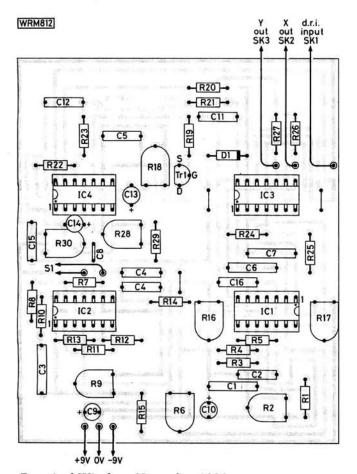
Fig. 5: Supply rail and de-coupling arrangements. Note that pin 7 of IC3 is not connected
