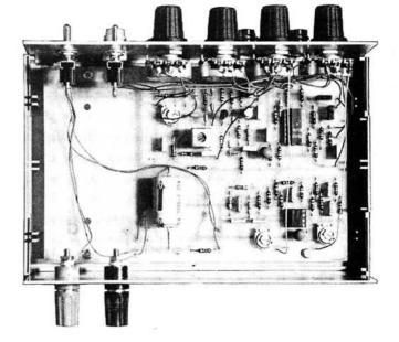
Photograph of the author's prototype showing the general layout of components
