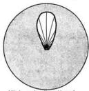
High gain directional two-element beam
