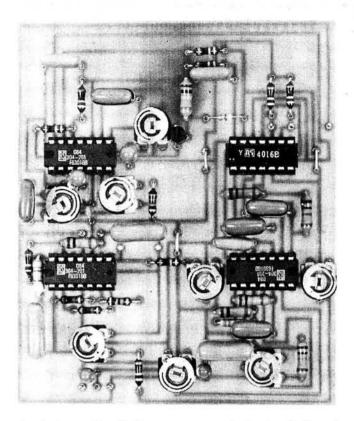
A photograph of the prototype d.r.i. circuit board which may be compared with Fig. 4
