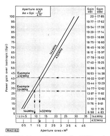
Fig. 10.4: The aperture areas for 144MHz and 432MHz antennas with the gain factors in dBd or dBi (right hand columns) and relative power gain over isotropic in the left hand (Y) column. Examples are shown with dotted lines
