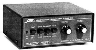
The AEA WB-1C is designed to be inserted into the  $50\Omega$  coaxial feeder between antenna and rig. It generates a steady stream of blanking pulses which control a gate in the antenna feed-line, isolating receiver from antenna when the pulse is present.
