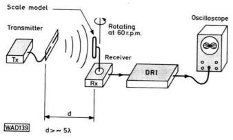
Fig. 1: The basic test set-up required to evaluate receiving transducers e.g. scale model antennas, directional microphones or photocells. The motor driving the model antenna rotates at the same rate as the d.r.i. scan. A full display will be provided on a high persistence or storage type oscilloscope
