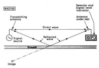
Fig. 10.1: Direct wave versus ground reflected wave from the signal source antenna to the antenna under test
