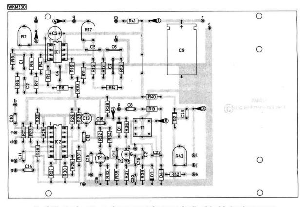
Fig. 2: The track pattern and component placement details of the i.f. signal generator
