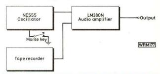
Fig. 1: Schematic block diagram of the training aid. The aim is to key the oscillator in time with the prerecorded input to develop correct style by direct comparison
