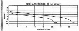
The voltage shown is plotted from the on-load voltage obtained at the end of each day's discharge (R20PP, power plus battery)
