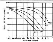
Performance as a function of temperature and load (Lithium/SO<sub>2</sub> battery)
