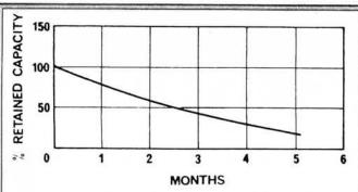
Charge retention with time for nickel-cadmium cells
