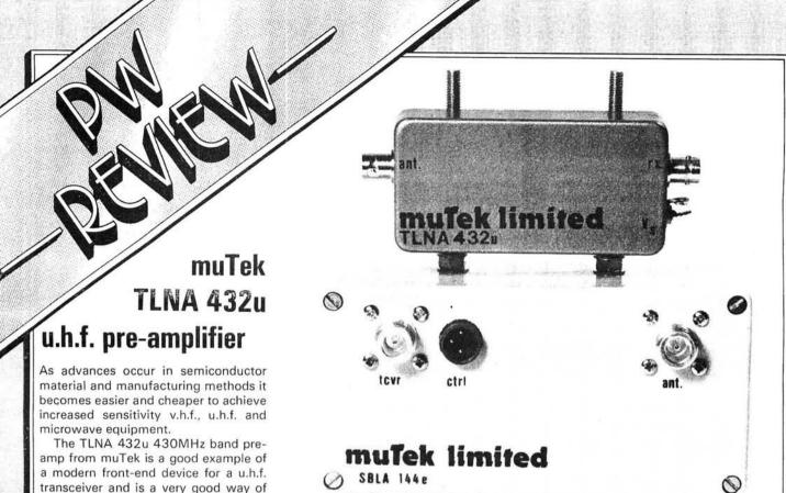
amp from muTek is a good example of a modern front-end device for a u.h.f. transceiver and is a very good way of updating existing 430MHz equipment, which is all too often not as sensitive as it could be. For an explanation of the effects of pre-amplifiers on equipment performance you are recommended to read the G3YGF article in the November and December 1981 editions of Radio Communication.
