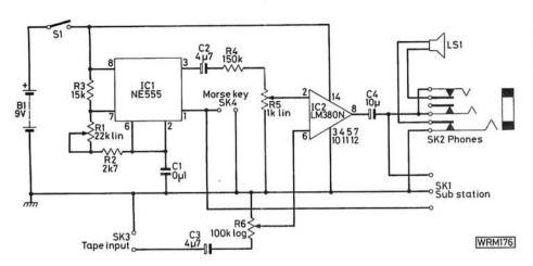
Fig. 2: Circuit diagram of the trainer together with details of the optional external substation. Pins 4 and 5 of IC1 are not terminated
