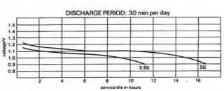
The voltage shown is plotted from the on-load voltage obtained at the end of each day's discharge (SP2 battery)
