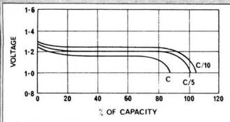
Capacity variation with discharge rate for nickelcadmium cells
