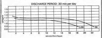
The voltage shown is plotted from the on-load voltage obtained at the end of each day's discharge (HP2 battery)
