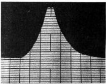
Fig. 4: Wideband response plot, centred on 145MHz, indicating the well-defined passband and excellent stopband characteristics. Horizontal axis 10MHz/div; vertical 10dB/div, input –20dBm
