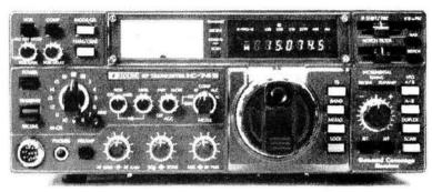
The IC-745's features include IF shift, 16 programmable memories with lithium battery back-up, passband tuning, a noise blanker both wide and narrow, threshold level control, notch filter, receive audio tone control and an all mode squelch. Also available is a front end switchable receiver preamp providing 12dB gain. RIT has a  $\pm$ 1KHz range.
