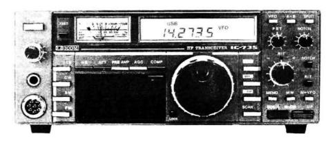
twin v.f.o.s, 10 memory channels (which include mode, frequency and offset information) and comprehensive scanning options. For base-station operation a d.c. power supply, desk microphone and external speaker are available together with the UT-23 speech synthesiser.
