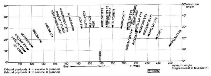
Fig. 2.2: The geostationary orbit as viewed from London
