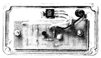
The author's prototype battery charger controller. The negative lead to the battery is bolted to the outside of the lid/heatsink
