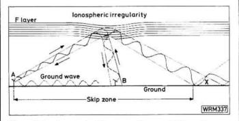
Fig. 8.1: Irregularities such as tilting in an ionospheric layer can cause scatter mode propagation so that signals from (A) arrive at some point (B) within a skip zone but which would otherwise only be heard at (X). Groundwave from (A) is too weak to reach point (B) This is because the signals may arrive at the point of reception from different directions which, in turn, will cause them to be randomly phased.
