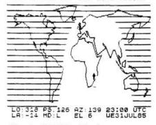
Fig. 1: OSCAR-10 close to apogee at 2300 on 31 July showing wide coverage (footprint) whilst transponder is on Mode "L"
