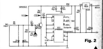
Note: The link should be connected to "a" when using the TTL output and pin 13 grounded using a through-board pin indicated on the p.c.b. layout. For the ECL outputs the link should be connected to "b" and pin 13 left open circuit
