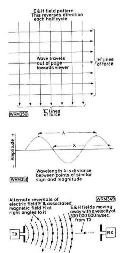
Expanding spherical wavefront note: At considerable distances from the radiator these appear as virtually parallel lines over small areas of space.
