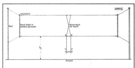
Fig. 3.8: Suggested constructional details of the Lazy H colinear broadside array
