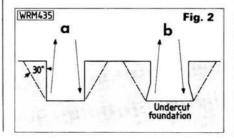
A suitable size of concrete block to enclose a tower of width 0.6m would be 1m square—which is about the smallest hole a man can dig without getting stuck on a pickaxe! If we dig a hole 1m deep and fill it with concrete, we will have 0.5 cubic m resisting uplift. In addition, an inverted half-pyramid of earth will help to resist uplift, its shape being determined by a 30° angle from the vertical at the bottom of the concrete block (Fig. 2(a)).
