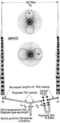
Fig. 3.1: Example Telex/Hygain system used to obtain endfire or broadside radiation from a pair of 18HT multi-band verticals
