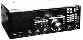
Continuous coverage from 150kHz to 30MHz. Two speed spin tuned VFO plus keyboard plus computer interface control.
