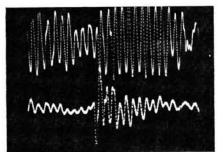
The boost in the average signal level of the processed signal (upper trace) is clearly shown in this 20ms snatch of speech
