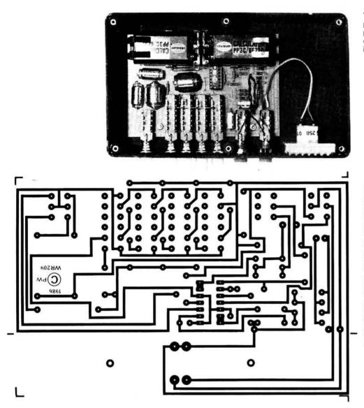
This photograph shows the p.c.b. fitted into a metallised plastics box. Any suitable size of box or case can be used, ideally though it should be metallic or metallised
