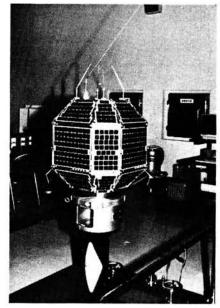
Fig. 5: JAS-1 under test
