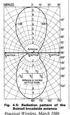
The Bobtail can also be constructed for other bands. The length of each half of the top line in metres can be obtained from
