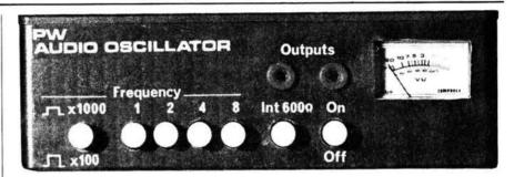
Front panel view of the completed oscillator. Round push-buttons have been used to simplify the cutting of the clearance holes in the panel
