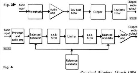
percentage copy in the presence of noise. The gain of the processor is then equal to this reduction. Under these conditions it was found that 4dB of gain was given using 15dB of a.f. clipping but using r.f. techniques only 10dB of clipping was required. By increasing the amount of clipping in both systems further gain was obtained, but using a.f. techniques the maximum gain which could be obtained was about 5dB whereas with an r.f. system in excess of 8dB was available.
