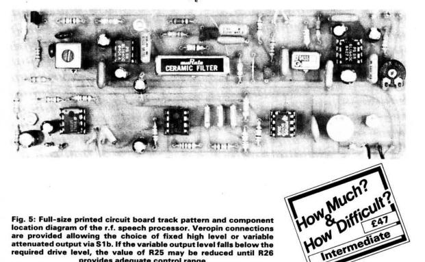
Fig. 5: Full-size printed circuit board track pattern and component location diagram of the r.f. speech processor. Veropin connections are provided allowing the choice of fixed high level or variable attenuated output via S1b. If the variable output level falls below the required drive level, the value of R25 may be reduced until R26 provides adequate control range
