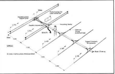
been reasonable, considerable DX has been worked with the antenna at only  $\lambda/2$  above ground and using 100W from the transmitter. In order to differentiate this antenna from its 144MHz counterpart it has been decided to refer to it as the ZL5-10.
