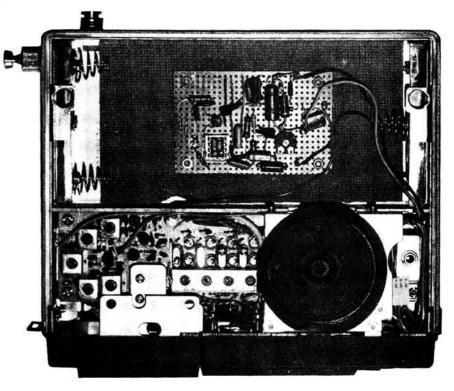
Prototype oscillator installed in IC-202E battery compartment
