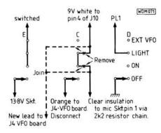
Fig. 4: Original function switch wiring and modification to 9V supply
