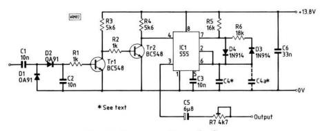
Fig. 1: Side-tone oscillator circuit
