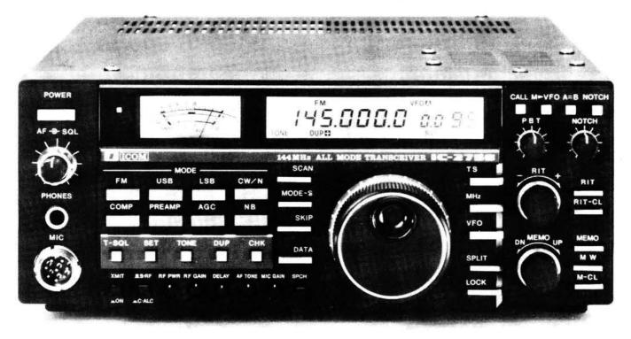
The ICOM IC-275E is the most advanced all-mode transceiver available to the Amateur today. It features a new technological breakthrough in frequency synthesizer sytems. This Direct Digital Synthesizer (DDS) operates in just 5 milliseconds, providing one of the fastest transceiver lock-up times available. Ideal for PACKET and AMTOR communication modes. The IC-275E has high sensitivity and dynamic range making it an ideal unit for contests and DX operation.
