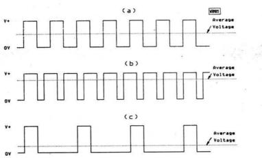
Fig. 1. The average output voltage from a non-retriggerable monostable is proportional to the input frequency
