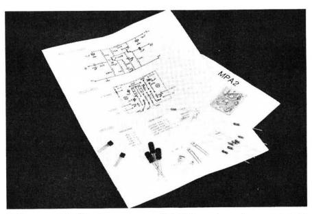
This month's kit is a very useful little microphone pre-amp from Wood & Douglas, the MPA-2. This is an improved version of their earlier and popular MPA1, the main difference being the addition of a buffered output. The unit's prime function is fairly obviously to boost the output of a low output microphone to a level suitable for feeding into a transmitter, as Elaine Richards G4LFM finds out.
