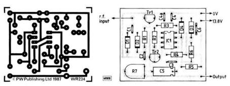
Fig. 2: Side-tone oscillator full size track pattern and component layout
