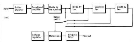
Fig. 2. Block diagram for the d.v.m. to d.f.m. converter
