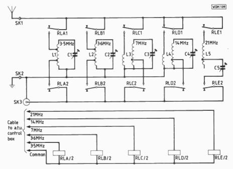
Fig. 2: Circuit diagram of remote antenna tuning unit
