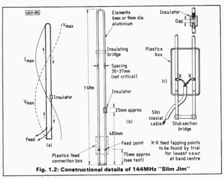
Unlike a "Slim Jim" for the 144MHz band, a strictly "frequency scaled" version for 28MHz, as above, would NOT be self supporting unless firmly secured to some form of base mount, preferably a quarter-wavelength above ground (at 28MHz) and then held vertical with insulating guy lines (polypropylene rope). The alternative is the thin wire version as in *Wires and Waves*.
