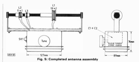
be covered when C2 is nearing minimum capacitance and resonates with L2 (l.w. coil).
