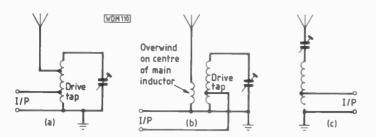
Fig. 3: Three basic tuning networks used by antenna tuning unit
