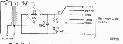
Fig. 5: Circuit diagram of power supply and control switch
