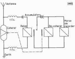
Circuit diagram of Marconi's test receiver
