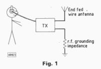
not be exceeded if your mains earthing and plumbing system are interconnected and your house is fed by an underground electricity service cable. For the 14MHz band and shorter wavelengths, most amateurs use either balanced antennas or quarter wave/ trapped verticals and radial earthing systems, not end fed wires. The effects of r.f. grounding impedance are likely to be encountered when working end-
