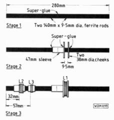
be obtained in the USA, at a high cost. However, they can be manufactured at home by taking two standard length ferrite rods and cementing them together end to end. In fact, the author has an experimental l.f. antenna using a rod some 480mm long, which may come as a bit of a shock to many readers.
