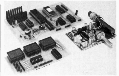
kit was to set the local oscillator frequency first, this should be 515kHz and can be measured at the test point. The output level at this test point is only a few millivolts and may be too low for use with a frequency counter, if this is the case then a good quality communications receiver tuned to 515kHz can be used.
