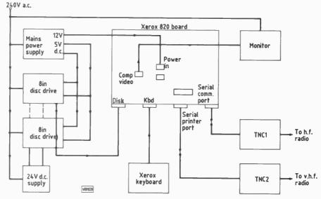
Fig. 1: The block diagram of the system. The heart of which is the Xerox 820 computer board with its power supply and keyboard. This was acquired from the States, kindly checked out by W3TMZ before being shipped to the UK
