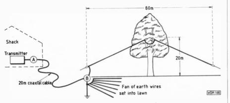
Fig. 1: Layout of author's all band long wire antenna Practical Wireless, July 1987
