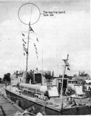
Fig. 1.4: Marine band "Slim Jim" mounted at the mast top of a renovated ex-WWII Motor Torpedo Boat
