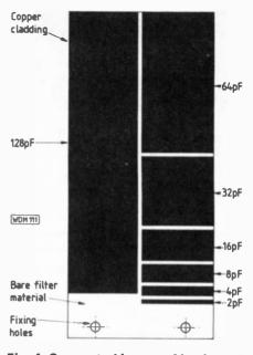
Fig. 4: Suggested layout of laminated p.c.b. capacitors
