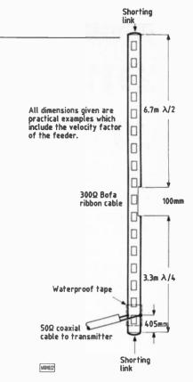
Fig. 3: "J-match" vertical for 21MHz band. Antenna can be supported in the same manner as  $5\lambda/8$  antenna
