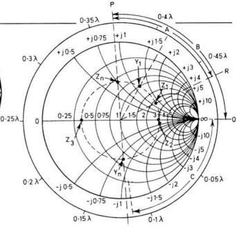
needed for a given reactance. For example, find the length of  $50\Omega$ cable having an inductive reactance of  $200\Omega$ .
