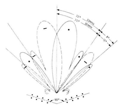
Fig. 1.6: The antenna pattern of the Knickebein array
