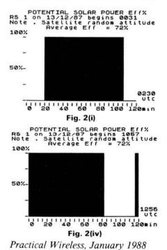
eclipse causing power exhaustion so severe that a full duration dash or dot could not be sustained, only permitting the tick of the make of the character before the power fell. The space between the pulses permitted enough charge to accumulate before the next "tick"
