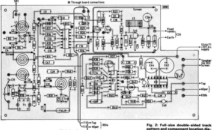
Fig. 2: Full-size double-sided track pattern and component location diagram of receiver
