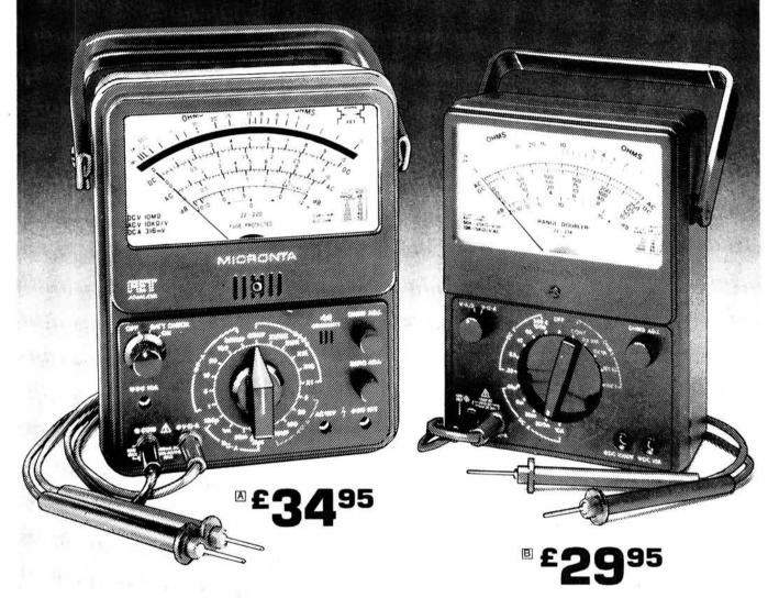
E 43-Range Multitester. 50,000 ohms per volt DC sensitivity. Fuse and overload protected. Measures to 1000 volts DC in 12 ranges and 1000 volts AC in 8 ranges. DC current to 10 amps, resistance to 20 megohms. Decibles: −20 to +62 dB. Requires one 9v and one "AA" battery. Measures: 6<sup>11</sup>/<sub>16</sub> x 4<sup>7</sup>/<sub>8</sub> x 2<sup>3</sup>/<sub>8</sub>".
