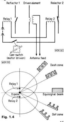
the dots and dashes were heard as a single note, thus telling the pilot he was on the correct approach. A simple presentation unit was also provided in the cockpit which showed the coursedeviation on a meter, and a form of range measurement was furnished by an S-meter arrangement.
