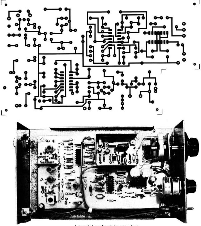
Internal view of prototype receiver
