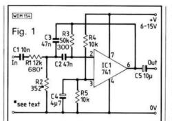
Note that the resistors R1, R2 and R3 are made up of two resistors in each case. See the text for further details
