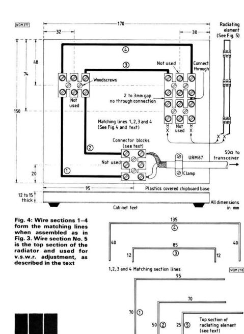
Fig. 3: Layout on baseboard of the matching lines which are comprised of (1 and 4) and (2 and 3) sections. Note the bottom of radiator element wires are secured at (X, X)
