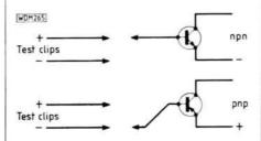
Fig. 2: Test connection details of npn and pnp transistors
