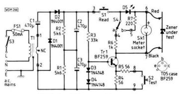
Fig. 1: Circuit diagram of Zener tester
