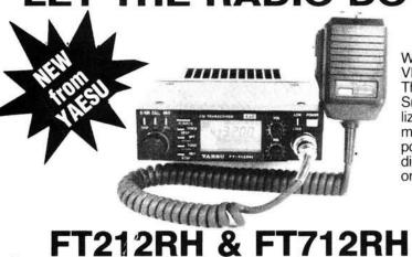
We are pleased to announce a new series of FM VHF and UHF mobile transceivers for the amateur. The 45/5W FT-212RH and the 35/4W FT-712RH. Smaller than their predecessors these models utilize a new cpu with greatly expanded features, most notable of which are 19 memories and support for the DVS-1 Digital Voice System, which can digitally record and playback from the microphone or the receiver.
