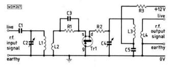
Fig. 6.1: The r.f. stage using a junction field effect transistor (j.f.e.t.)
