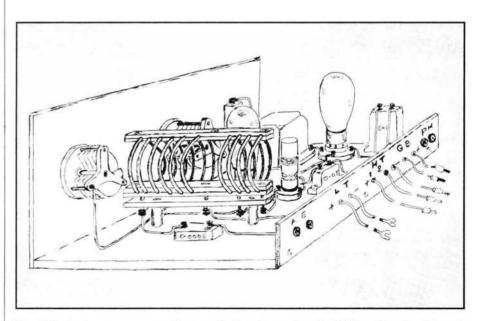
Fig. 1.2: A short wave receiver made by the author in 1935 using the "bread board" design. The valves had 2 volt heaters and together with other components were salvaged from old domestic radios, and the plug-in tuning coils were home made.
