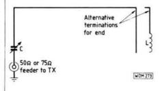
Fig. 2.4: The  $\lambda/3$  antenna, successfully used by the author on Top Band
