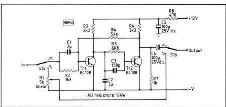
Fig. 1: The circuit of the converter
