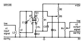
Fig. 6.3: A regenerative detector using a dual-gate m.o.s.f.e.t.
