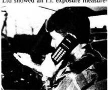
ment system from the US manufacturer Holaday Industries Inc. The 6-minute averaged value required to meet the ANSI (American National Standards Institute) exposure standard is calculated by the built-in microprocessor and is displayed by an l.c.d. readout which is updated every five seconds. Accurate time-averaged readings can be important for those who climb through the high-field regions of transmitter towers.
