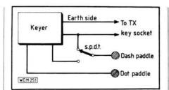
Fig. 1: The wiring in of the singlepole two-way switch that transforms your Morse key
