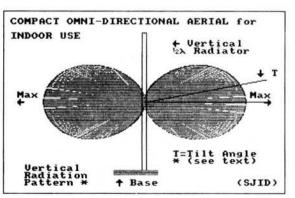
Fig. 2: Vertical radiation pattern of the compact indoor antenna. See text regarding "tilt" angle
