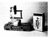
Fig. 2.4: Replica of the original microphone invented by Professor Hughes (circa 1850)
