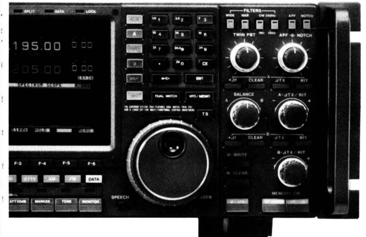
The IC-781 has a dual-watch function which allows simultaneous receive of two frequencies in the same band. Balance controls adjust VFO A/B receive strength levels. This feature is especially useful on Dx-expeditions or contests to check band activity or to tune in your next contact. The newly developed ICOM DDS (Direct Signal Synthesizer) system is incorporated to provide a fast transceiver lock-up time. This is essential for data communication systems.
