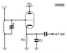
Fig. 1.2: The basic infinite impedance detector
