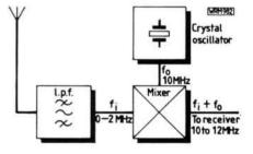
Fig. 1: Block diagram of converter
