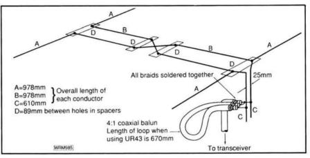
Fig. 1: Main antenna elements are made from pvc insulated conductors stripped from either 1.00mm<sup>2</sup> or 2.5mm<sup>2</sup> twin and earth mains cable
