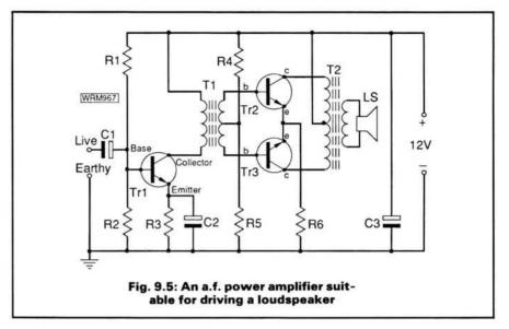
gets its name from the way the circuit operates. During the half-cycle that the base of Tr2 is being driven positive, the base of Tr3 is being driven negative. Whilst one transistor is "pushing" the other is "pulling". Similarly, the collector of Tr2 will reach a negative peak at the same instant that the collector of Tr3 reaches a positive peak.
