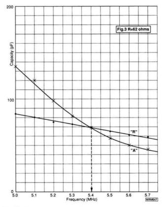
Fig. 3: Shows variation of the capacitor in the matching unit with antenna connected "A", and with resistor connected "R". The resonant point is at 5.4MHz
