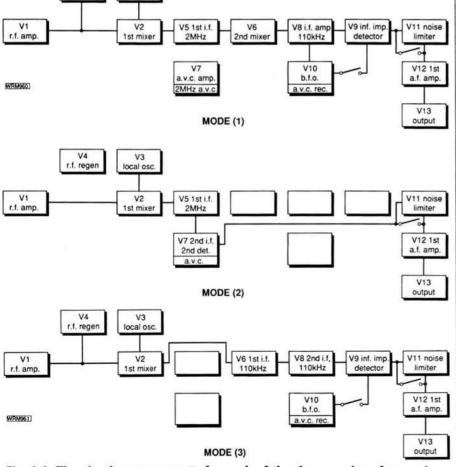
Fig. 1.1: The circuit arrangements for each of the three modes of operation, simplified to block diagram form
