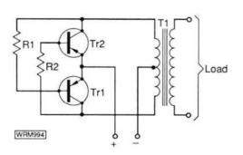
Fig. 1: Basic asynchronous d.c. to a.c. converter circuit
