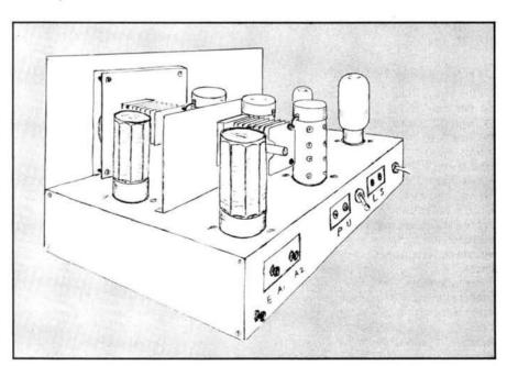
Fig. 5.2: The 2V2 All-mains short wave receiver
