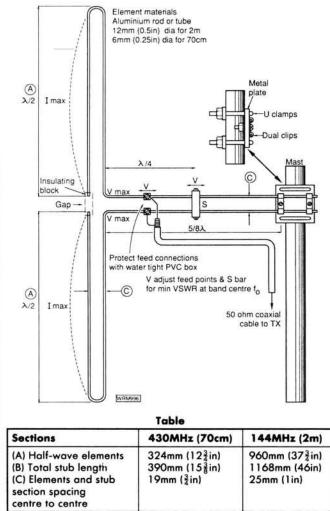
Tolerances: (A) For 70cm:  $\pm$  3mm ( $\frac{1}{8}$ in). For 2m:  $\pm$  6mm ( $\frac{1}{4}$ in) (B) Must be as exact as possible (C) For 70cm and 2m: ±3mm (1)in)
