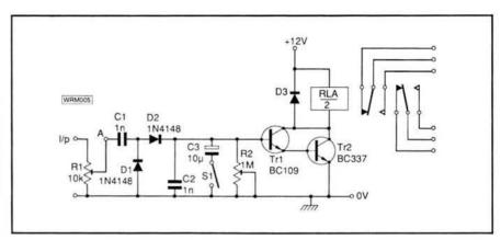
Fig. 1: Basic circuit of r.f. operated relay. D3 is a 1N4005
