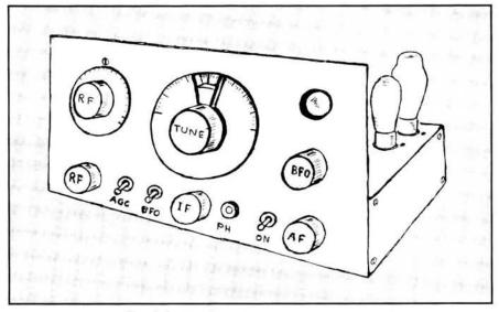
Fig. 6.2: The Superheterodyne receiver
