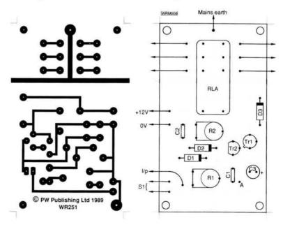
Fig. 2: Full size single sided track pattern and component placement diagram. Note, mains earth connection need only be used when the relay is controlling mains powered equipment
