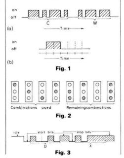
or ITA 2, the letter "A" would be represented by the first two lamps being on and the last three being off. Similarly, every other letter of the alphabet is associated with a different, unique combination of "on's" and "off's". To send "A" using the ITA 2 code we simply decide the length of a "bit", turn on the carrier for twice this period and then turn it off for three times this period, see Fig. 1(b).
