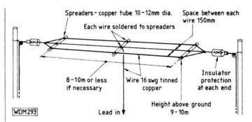
voltage reading has remained virtually constant, showed the tinned copper wire antenna to have a pick-up efficiency far, far greater than the one made from covered wire.
