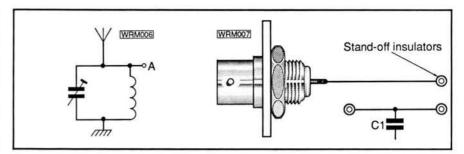
Fig. 3: Tuned circuit for making the r.f. relay frequency-selective
