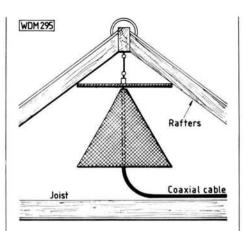
Fig. 4: Typical roof installation of antenna
