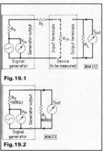
to high across the spectrum where the filter is expected to operate, whilst maintaining the input level indicated by the voltmeter  $V_{in}$  at a constant level, noting any changes in the reading of the voltmeter  $V_{out}$  across  $R_L$ . Plotting output level against frequency on graph paper will give the frequency response of the filter being tested.
