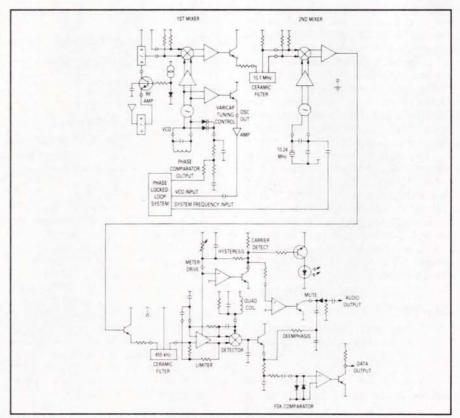
Fig. 1: Internal block diagram of MC3363
