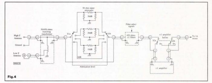
steps of 5dB) for impedances of 50, 75 and  $450\Omega$  are catered for. Other level of attenuation can be worked out from the formula already given. As well as the exact resistor values, rounded values are also given. In practice, the rounding of these values makes very little difference to the performance of the attenuators.
