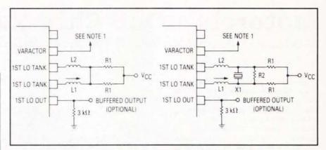
Fig. 2: Alignment circuit for first local oscillator
