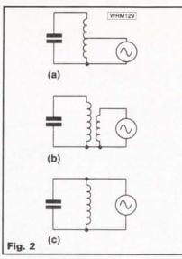
usually specified but often shown as a proprietary makes. These were known as "Hi Q" dust cored coils, which of course, have a higher Q than a similar dimensioned device without core. However, just out of curiosity I tried a home-made coil, say 50mm dia x 76mm long of 20 s.w.g. wire and the improvement must be heard to be believed.
