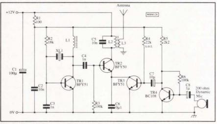
Fig. 1: Circuit diagram of the experimental transmitter 48
