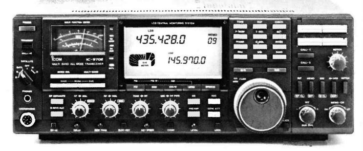
Designed for the serious operator on the 144, 430 and 1200MHz bands, Icom's new IC-970E has up-to-date technology for DX, digital and satellite communications.
