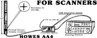
The **HOWES AA4** Active Antenna gives full coverage from 25 to 1300MHz. It is designed to be the ideal solution for those requiring a compact, broadband antenna for use with scanning receivers. The AA4 features advanced technology with a low noise microwave IC amplifier.
