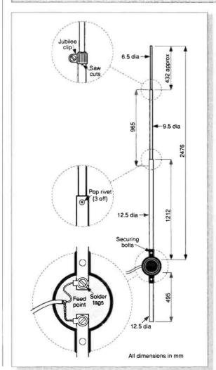
Fig. 1: G4XPP's simple antenna design
