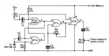
Fig. 1: The circuit, based on a single c.m.o.s chip and a few other components.
