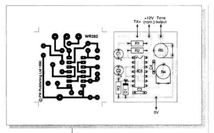
Fig. 3: The board and component overlay. Small enough to fit into almost any rig without a repeater access oscillator.
