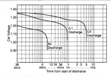
Fig. 1: Terminal Voltage curves for NiCad cells for various discharge periods.
