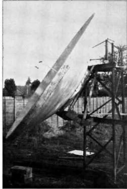
tropo system has to be dismantled and moved up the garden taking about two hours to set up.
